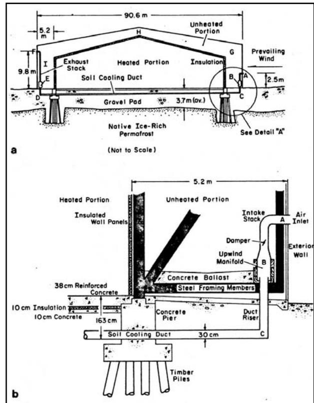
Figure 2. a) Hangar Cross-section b) Detail of pile system and air duct system. (Tobiasson 1973)
