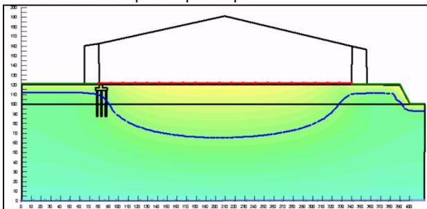
Figure 5. Thaw depth extent estimation utilizing Temp/W commercial software. 0°C isotherm after 25 years of heated hangar operation. Figure axes in feet
