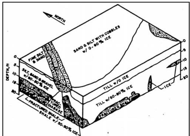
Figure 3. Isometric diagram of the soil conditions beneath Hangar 10. Note the massive ice in the northwest corner and bedrock at 3 m depth. Figure units in feet. (Tobiasson 1970).
