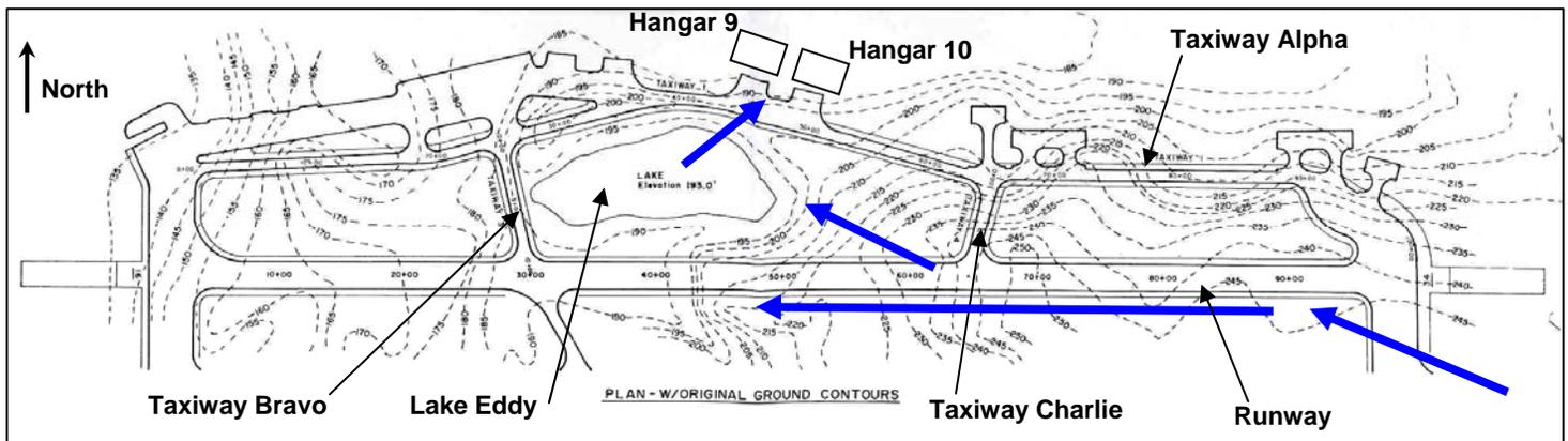
Figure 4. Area map. Bold arrows indicate water flow paths. Preconstruction contours in feet.
