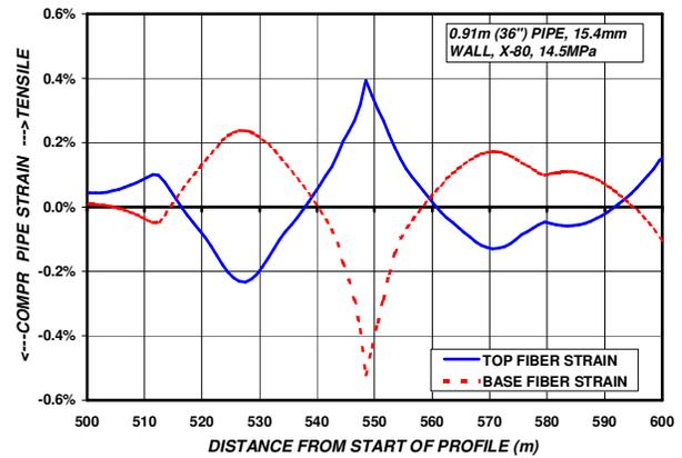
Figure 12. Close-up pipe strains near high settlement area
