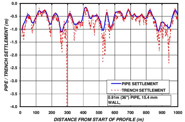
Figure 9. Predicted pipe and soil displacements
