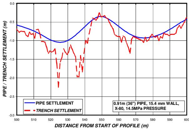
Figure 10. Close-up of pipe and soil settlements
