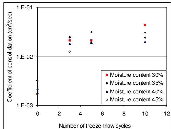
Figure 5. Coefficient of consolidation with number of freeze-thaw cycles for samples from I site
