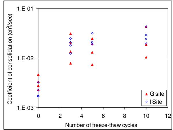
Figure 9. Coefficient of consolidation for samples from I and G sites
