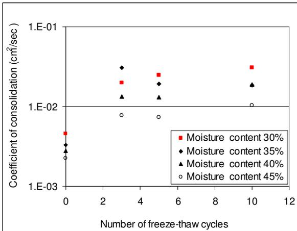
Figure 7. Coefficient of consolidation and number of freeze-thaw cycles for samples from G site
