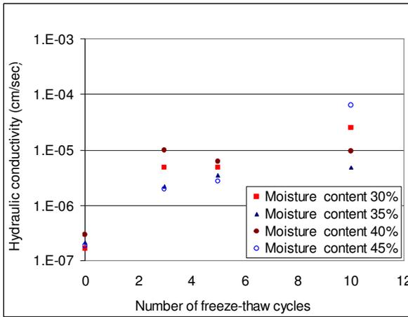
Figure 8. Hydraulic conductivity and number of freeze-thaw cycles for samples from G site
