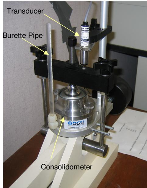
Figure 4. Testing arrangement for coefficient of consolidation and hydraulic conductivity
