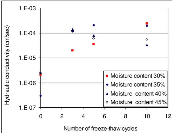
Figure 6. Hydraulic conductivity and number of freeze-thaw cycles for samples from I site
