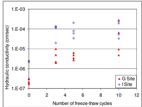
Figure 10. Hydraulic conductivity of samples from I and G sites
