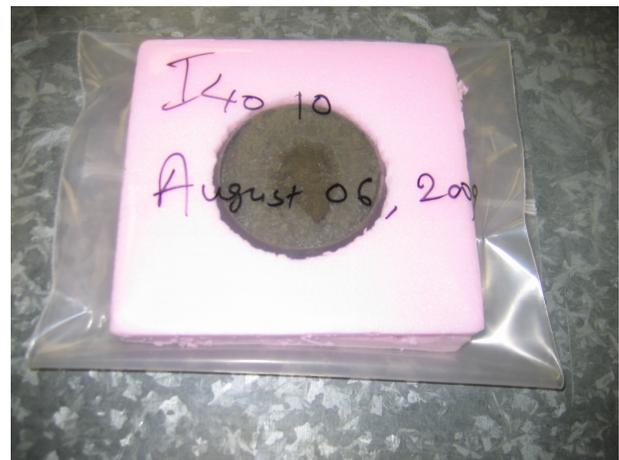
Figure 3. Sample assembly with insulation for one-dimensional freezing and thawing
