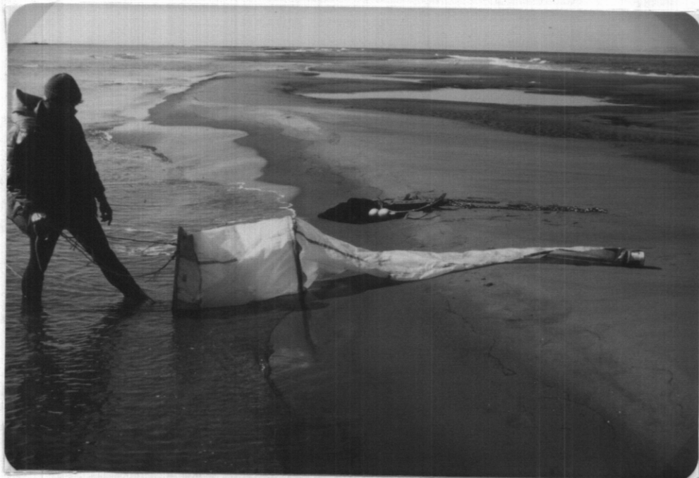
PLATE 3. Modified Faber net pelagic trawl for sampling zooplankton and pelagic fish larvae.
