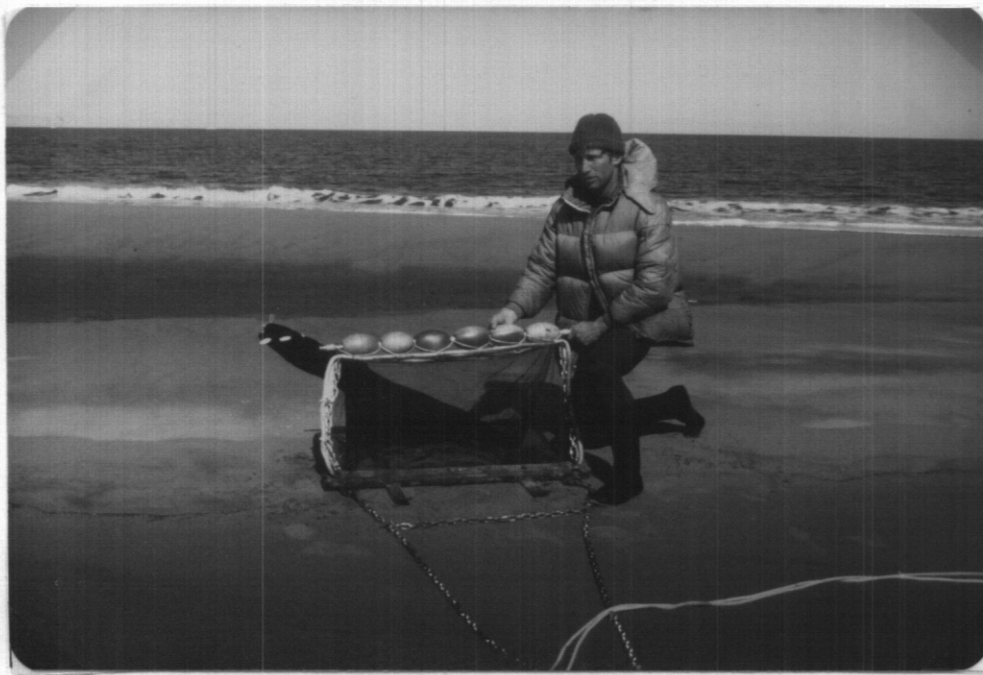
PLATE 2. Epibenthic trawl used for sampling bottom-dwelling macroinvertebrates and fish.
