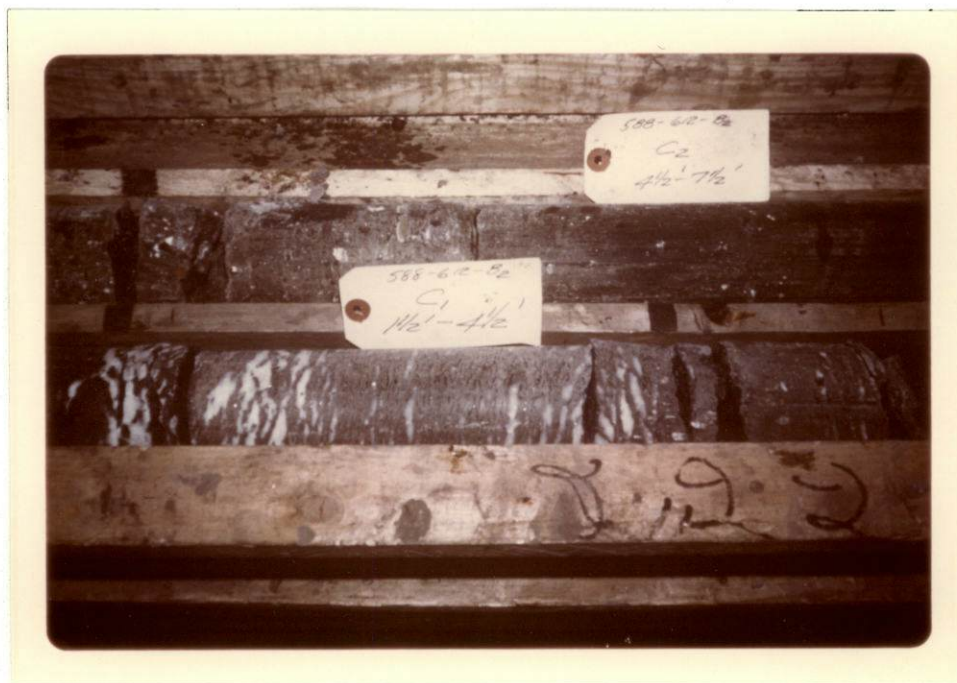
Photograph 22: Clay till cores from Test Hole 612. Observe the ice banding in the lower sample in this photograph.
