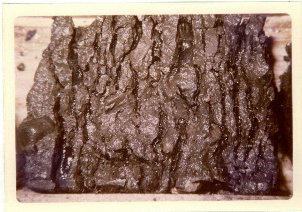
Photograph 36: A close-up of the sample shown in Photograph 35. This photograph is approximately full size. Notice the ice lenses and the pebbles within the material.
