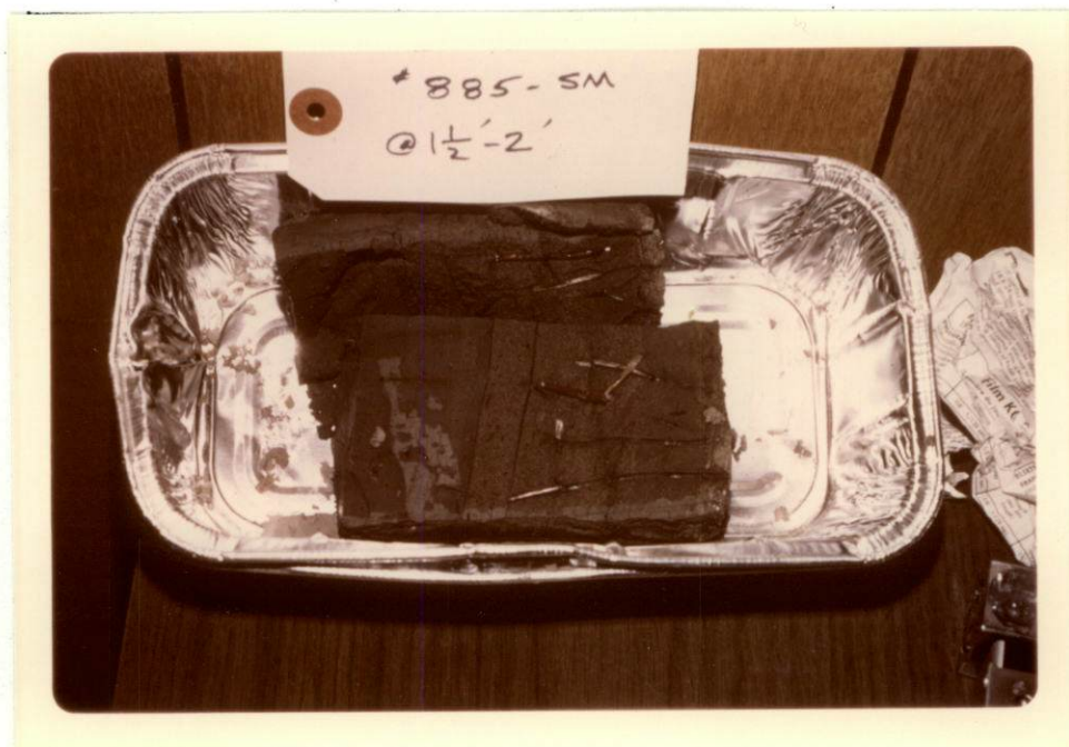
Photograph 26: A sample of organic silt from Test Hole 885 at a depth interval of 1.5 to 2.0 feet. Note the organic material.
