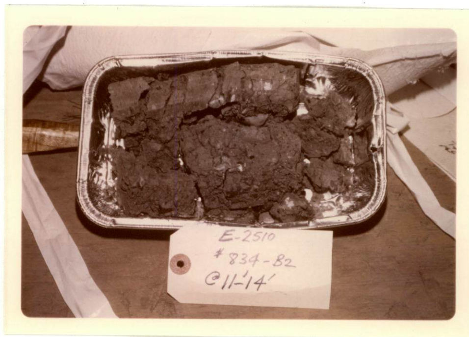
Photograph 24: A sample of clay till, silty-sandy, water content 9 percent, from Test Hole 834 at a depth of 11 to 14 feet. Note there is no visible ice in this sample.
