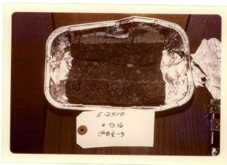
Photograph 30: A sample of silty-clay, medium plasticity, from Test Hole 916. Note the pebbles within this material. Water content was 25 percent.
