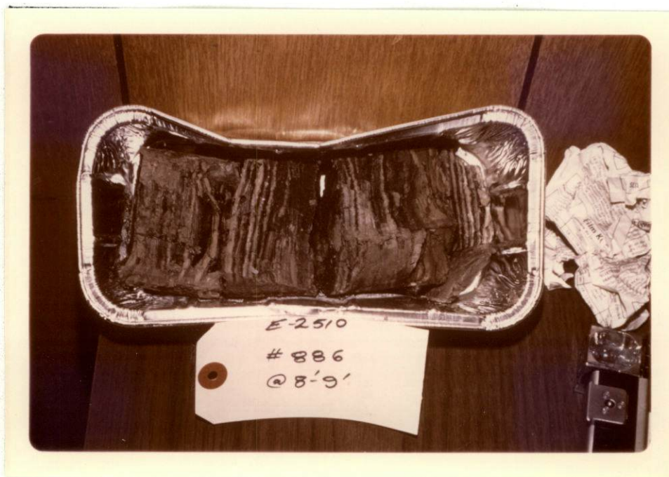
Photograph 28: A sample of varved clay from Test Hole 886. This material was laid down in still water and the light and dark bands are alternating layers of silt and clay. Water content of this material was 28 percent.
