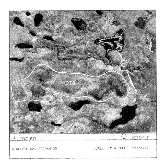
general fill. The site has a moderately high environmental sensitivity rating. Access to the site crosses thermally sensitive terrain thereby necessitating winter operations. Haulage distance to proposed construction sites is reasonable. Site 1078 has a good potential as a source of shale borrow material.
