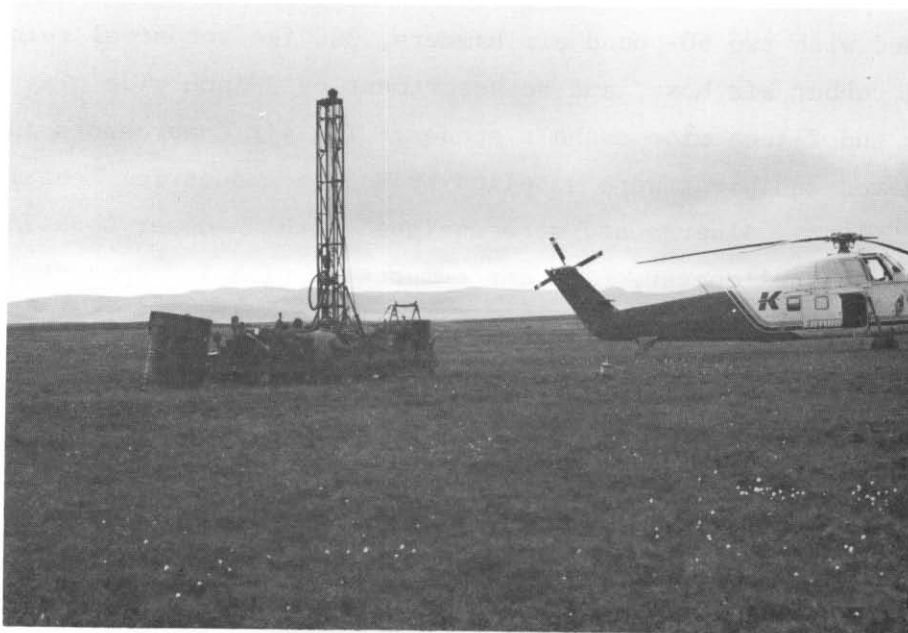
Photo 3.1.1 View of Kenting Big Indian Heli-Drill drilling by means of airflush to prove out depth of granular materials deposit on the Yukon coastal plain.
