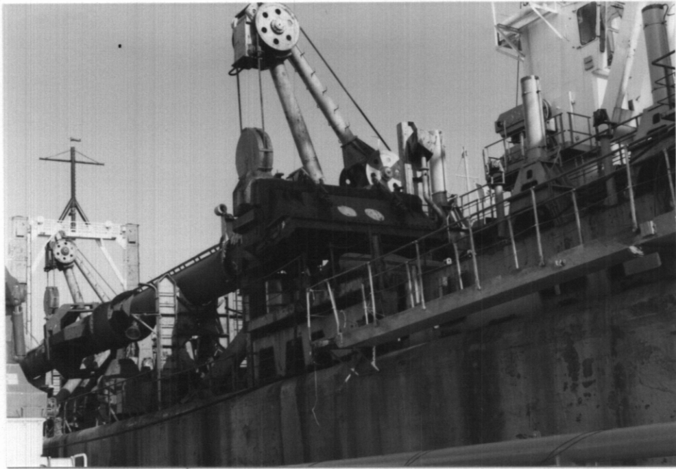
Plate 1. View of draghead and suction pipe stored in davits aboard the hopper dredge "Geopotes X".
