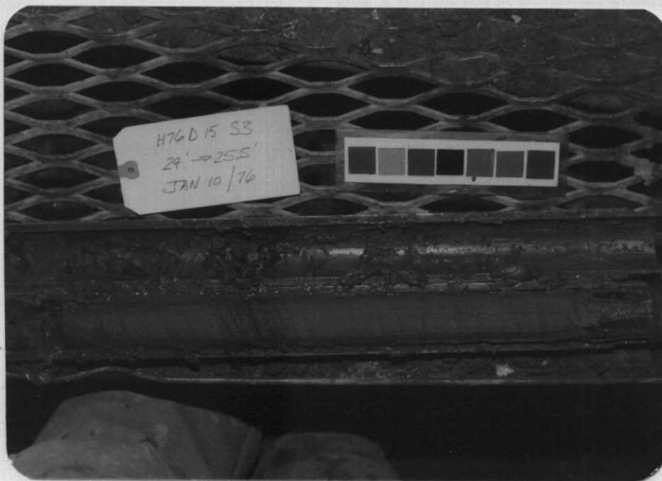
PHOTOGRAPH No.2 Typical Split-Spoon Sample (from Dock Site H76-D15)
