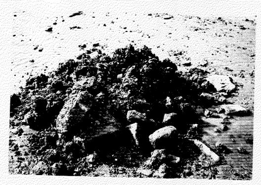
Coarse sediments from to 0.7 meters at test pit 235 - 01 - MB. Tidal currents significantly affect the size, sorting and distribution of sediments over most of the tidal flats.
