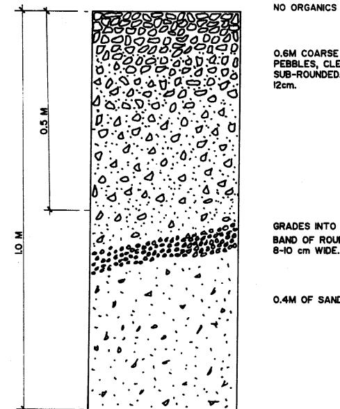
O.6M COARSE GRAVEL AND PEBBLES, CLEAN, ANGULAR, SUB-ROUNDED. MAX. SIZE 12cm.
