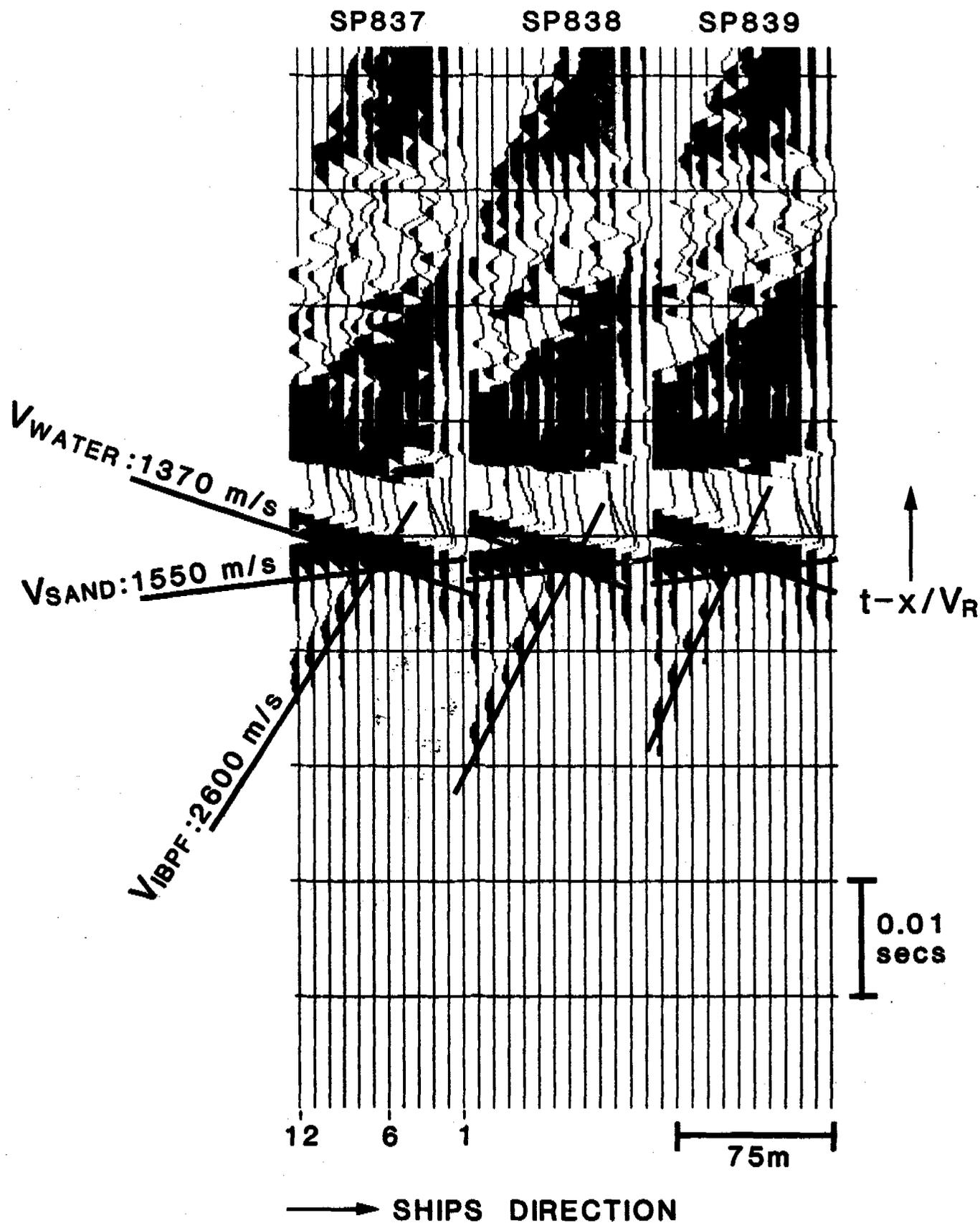
FIG. 4 12-CHANNEL SEISMOGRAMS; "REDUCED TRAVEL TIME".
