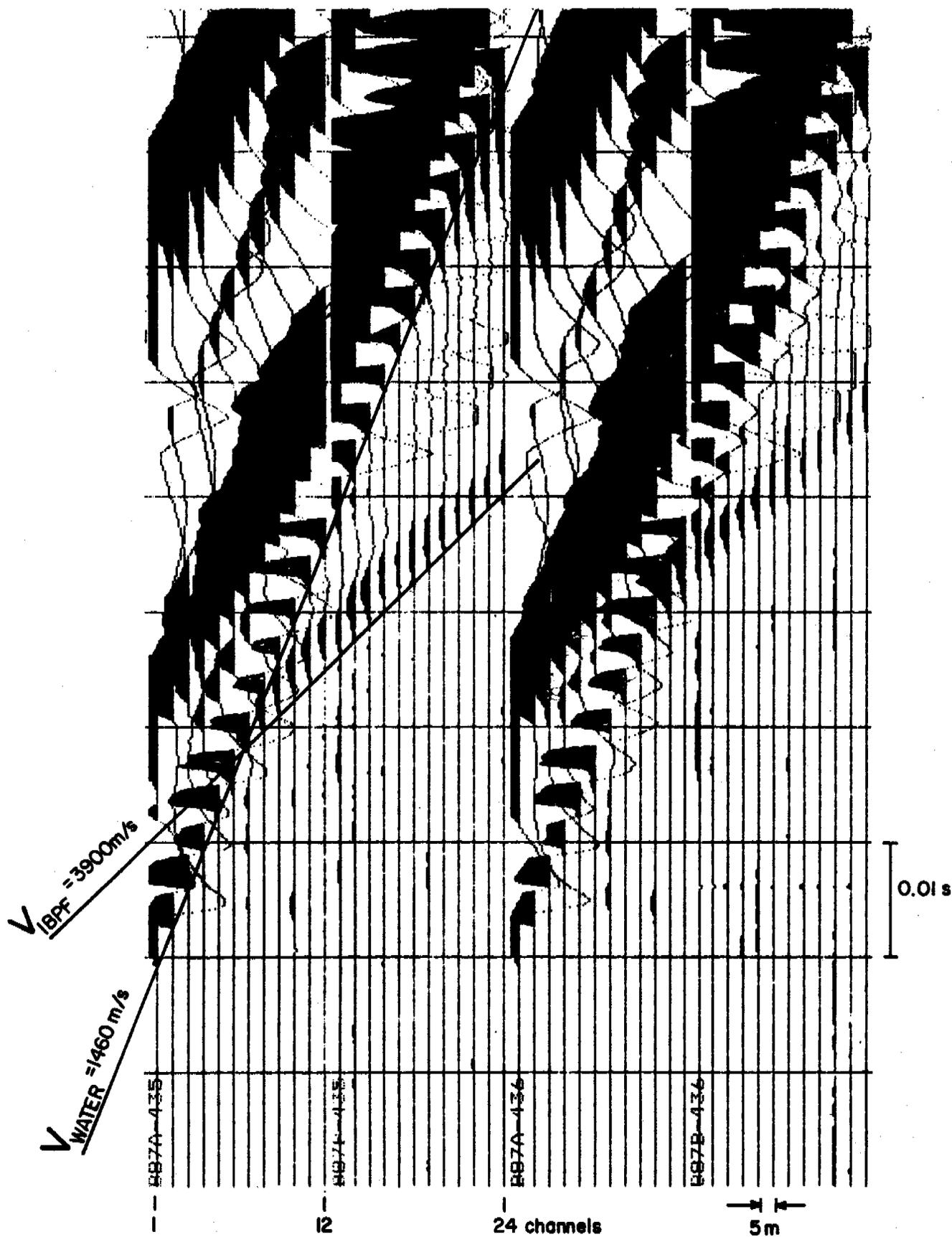
FIG. 5 SEISMOGRAMS SHOWING REFRACTED EVENTS ASSOCIATED WITH ICE-BEARING PERMAFROST (IBPF).
