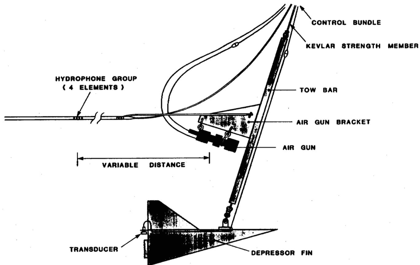
FIG. 3 FORWARD UNIT OF THE EEL.
