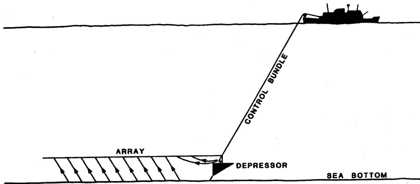
FIG. 2 DEEP-TOW REFRACTION ARRAY.
