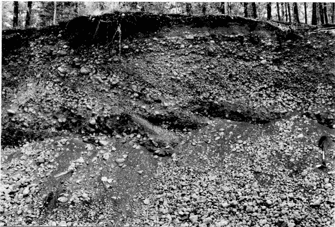
Photo 6: Bedding and gradation at NWT highway pit, Salt Mountain. Note sandy lenses and variation in size of rocks.
