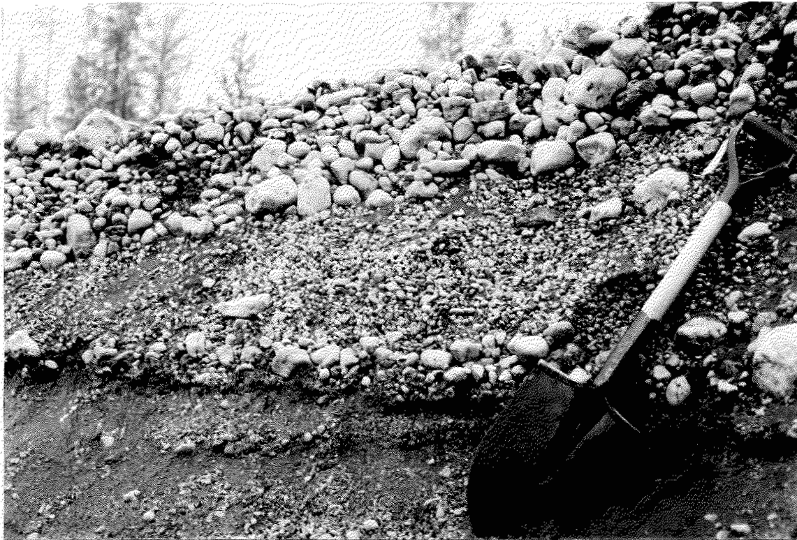
Photo 5: Bedding and gradation at NWT highway pit, Salt Mountain. Note abundance of limestone and dolomite rocks.
