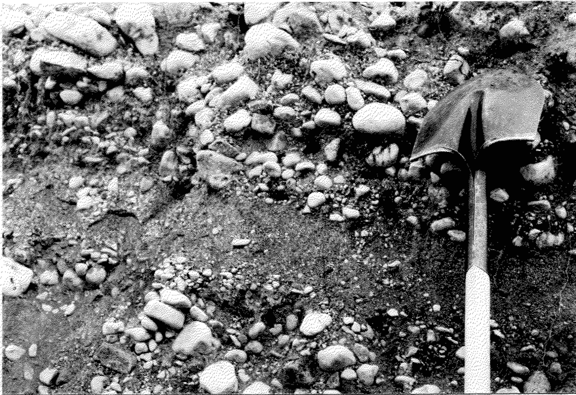
Photo 7: Gravels in Pit 2, site of Sample 3. Note well rounded clasts, abundance of limestone and dolomite rocks, bedding structures and general gradation contrast among different beds.
