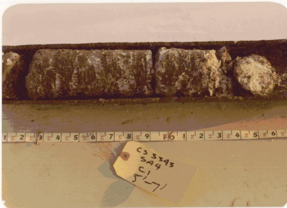
PHOTOGRAPH No. 5 Typical CRREL Core of Ice-rich Soil on Airstrip.
