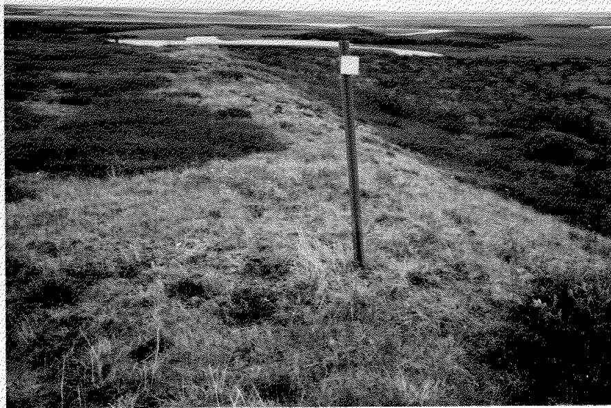
Photo 6. Angle iron and identifying plate marking location of survey post established as a reference point for future surveys along Ya-Ya esker complex.
