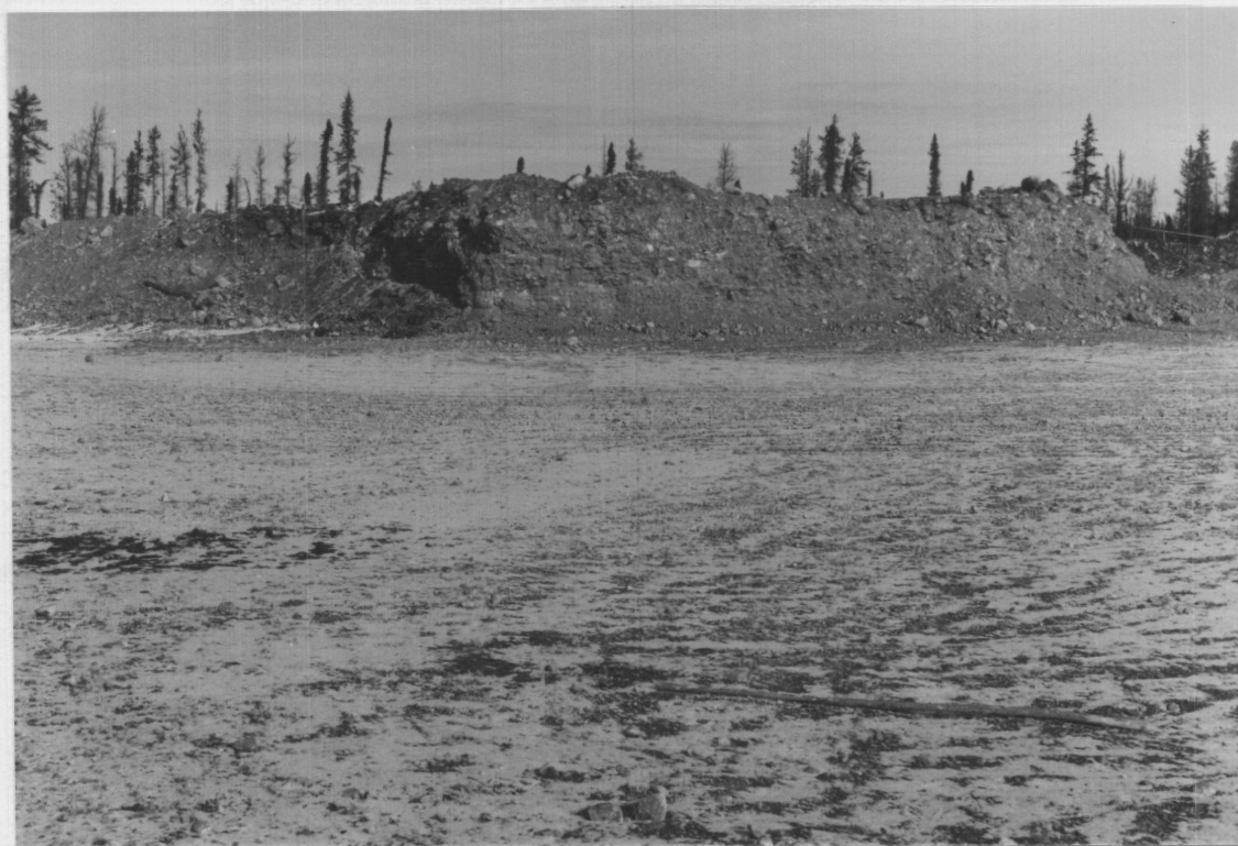
11. Deposit 5-6 (HR-109A): View of north side of recently-excavated pit, showing cobbly, relatively poorly graded, aggregate in upper section of deposit.
