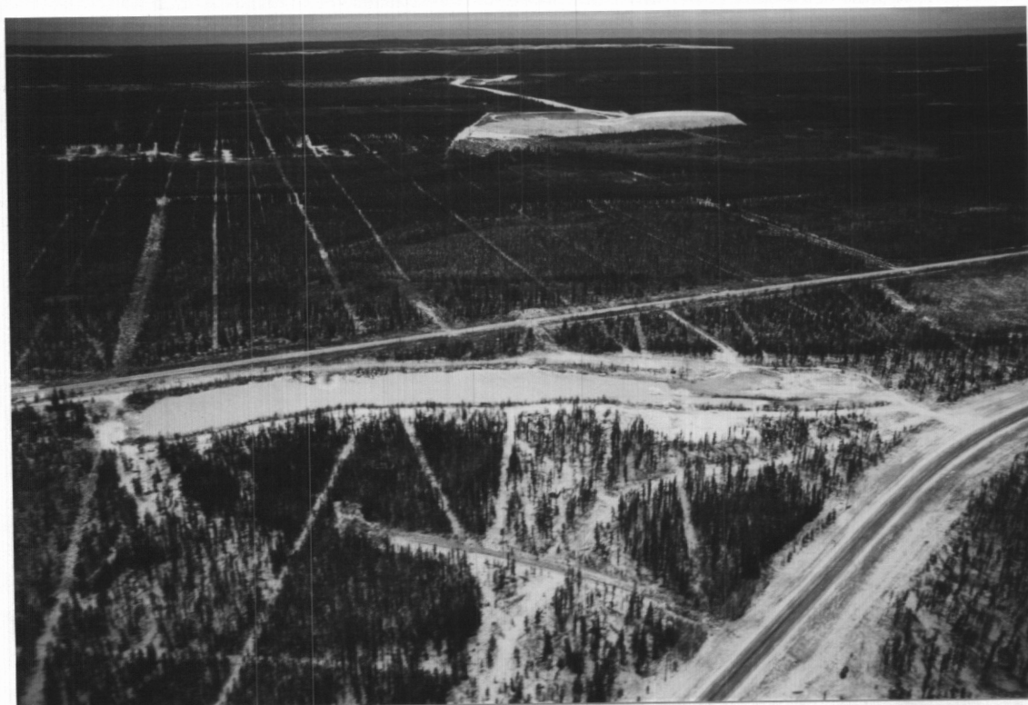
PHOTO 46: Roadside borrow pit at east end of Deposit 6-3. A mine waste dump (possible future source of Class 5 aggregate) is visible in background.
