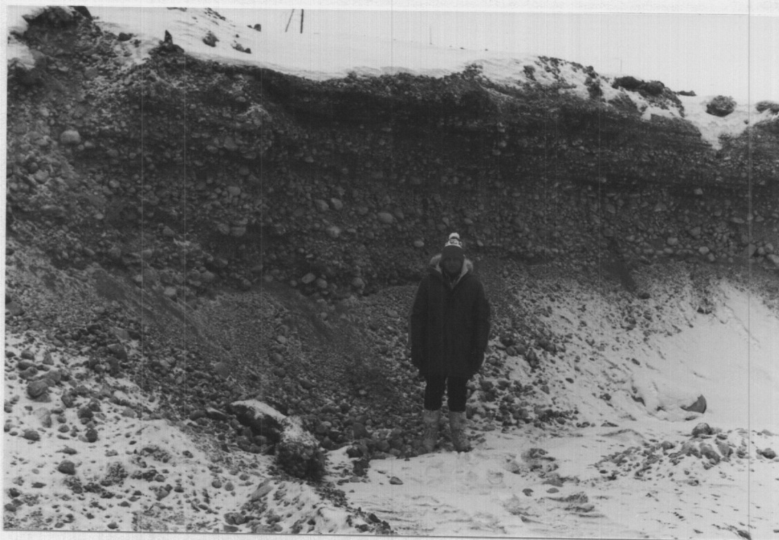
25. Deposit 5-40 (km 64.5): South end of recently developed pit, exposing about 2.5 m of moderately to well graded coarse aggregate.
