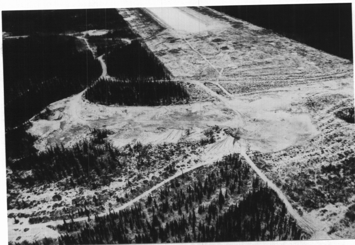
PHOTO 55: Deposit 6-22, comprising lag gravel deposits on bedrock high, is located at north end of Fort Resolution airstrip.
