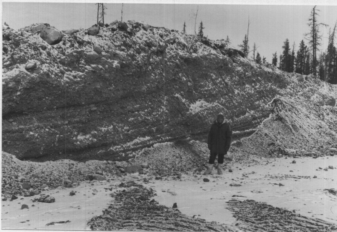
19. Deposit 5-14 (HR-124A): northeast corner of recently developed pit. 2.5 m to 3 m of gravel has been removed down to the underlying clay till.
