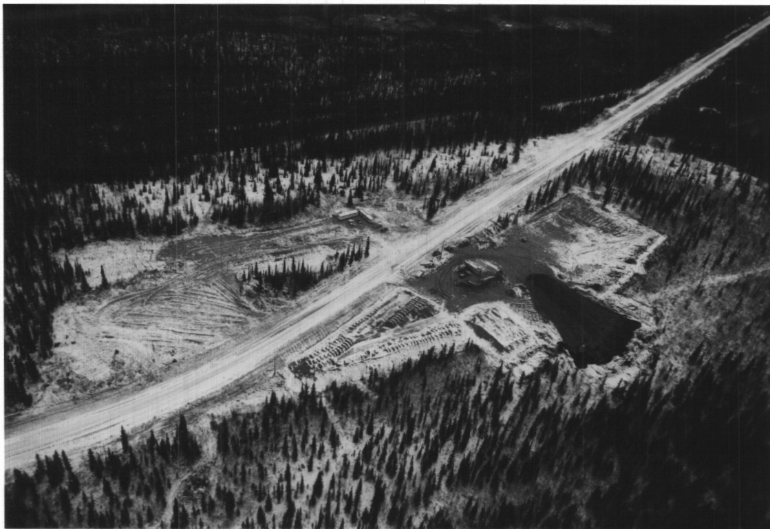
PHOTO 53: Active pit area, Deposit 6-20. Material is being extracted for use in highways maintenance.
