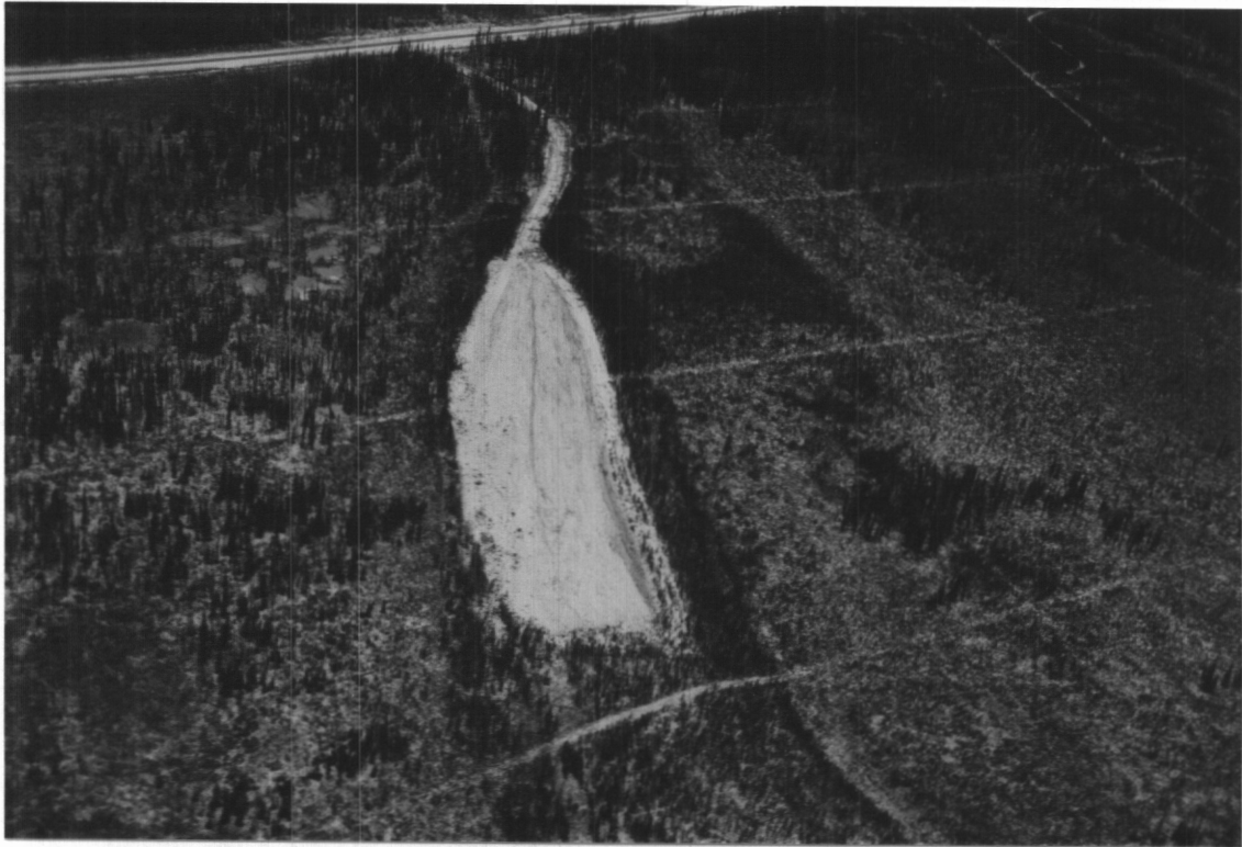
PHOTO 41: Abandoned pit area, Deposit 5-39. Existing pit appears to be depleted; however, considerable material remains further to the east.
