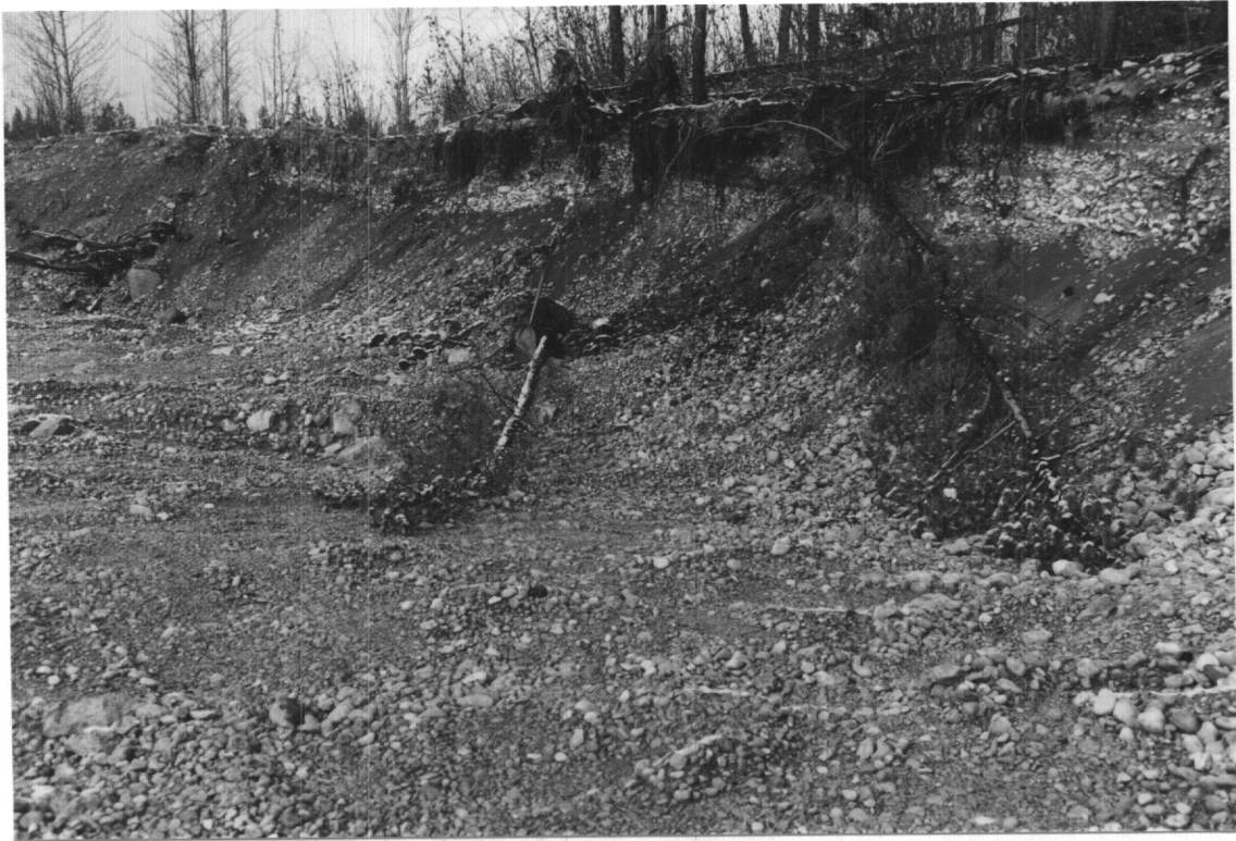
PHOTO 5: Salt Mountain South Pit, Deposit 5-69. Coarse, gap graded, sand and cobble material is exposed along east wall of pit.
