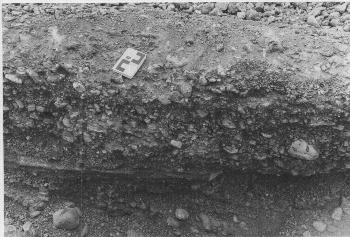
32. Poorly-graded gravel exposed in shallow road-side pit, Pine Point Mines.
