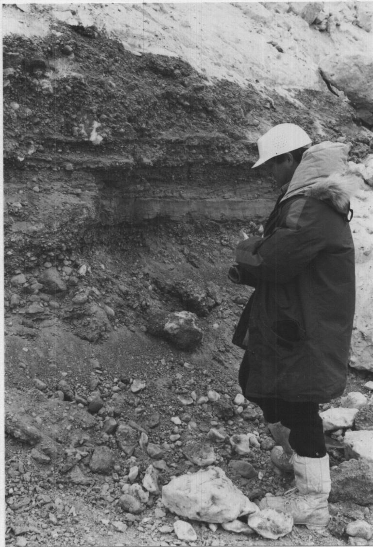
33. Poorly graded aggregate exposed in road fill pit east of Pine Point Mines plant site.
