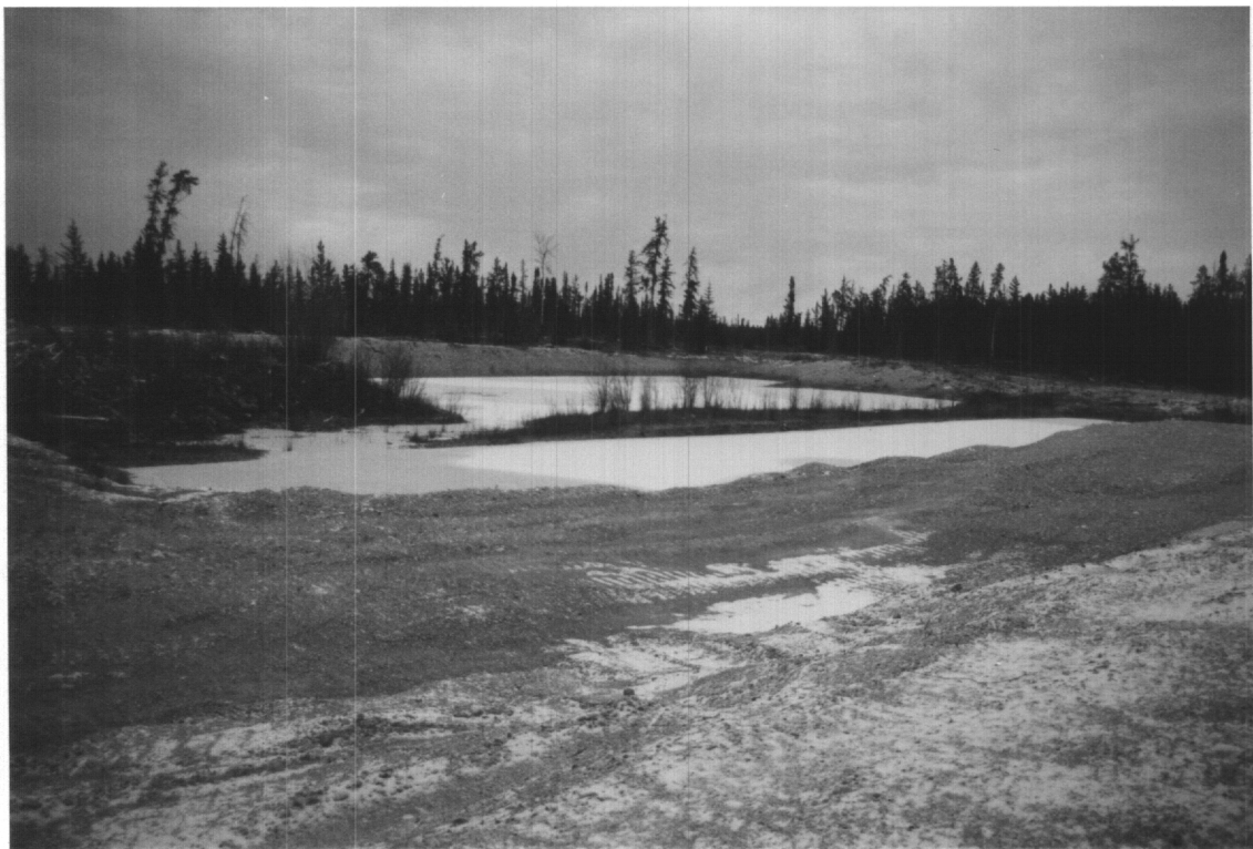
PHOTO 38: Pit area, Deposit 5-33. Note that material thickness above the water table is only about 1 m. It is understood that aggregate is extracted from below the water table for use in concrete.
