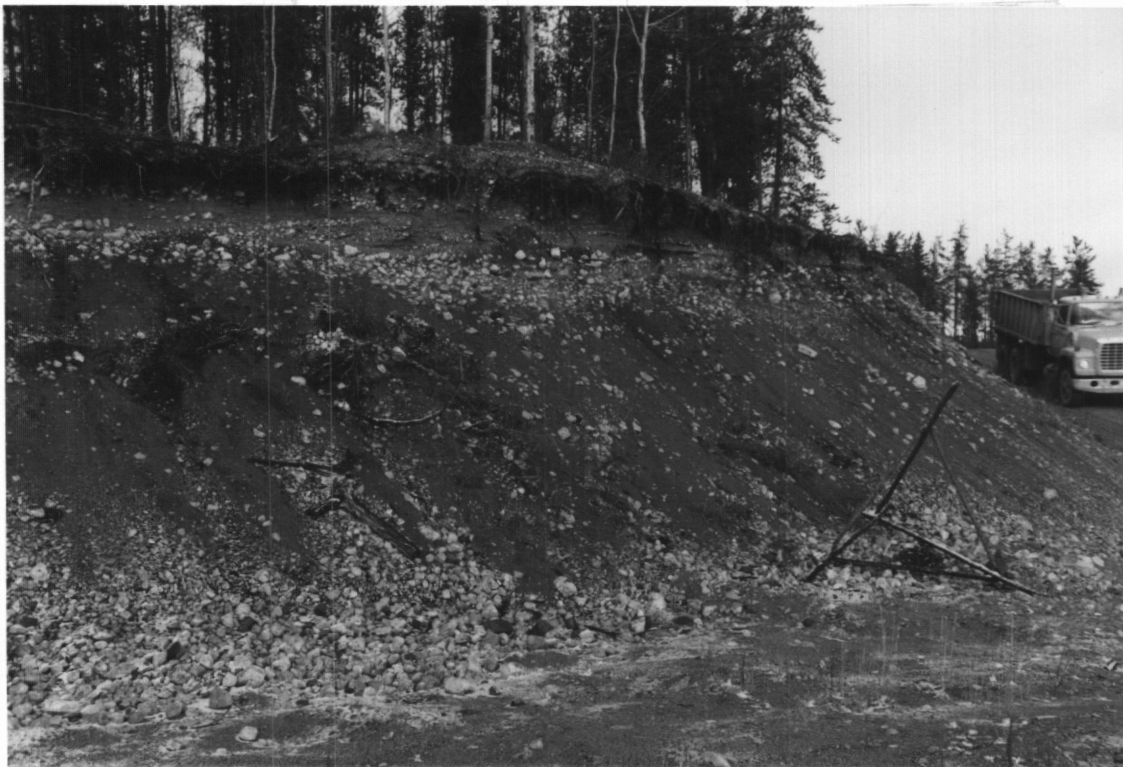
PHOTO 10: Salt Mountain DPW Pit (Km 232.5), Deposit 5-70. Exposure along north pit wall shows typical sandy gravel material.
