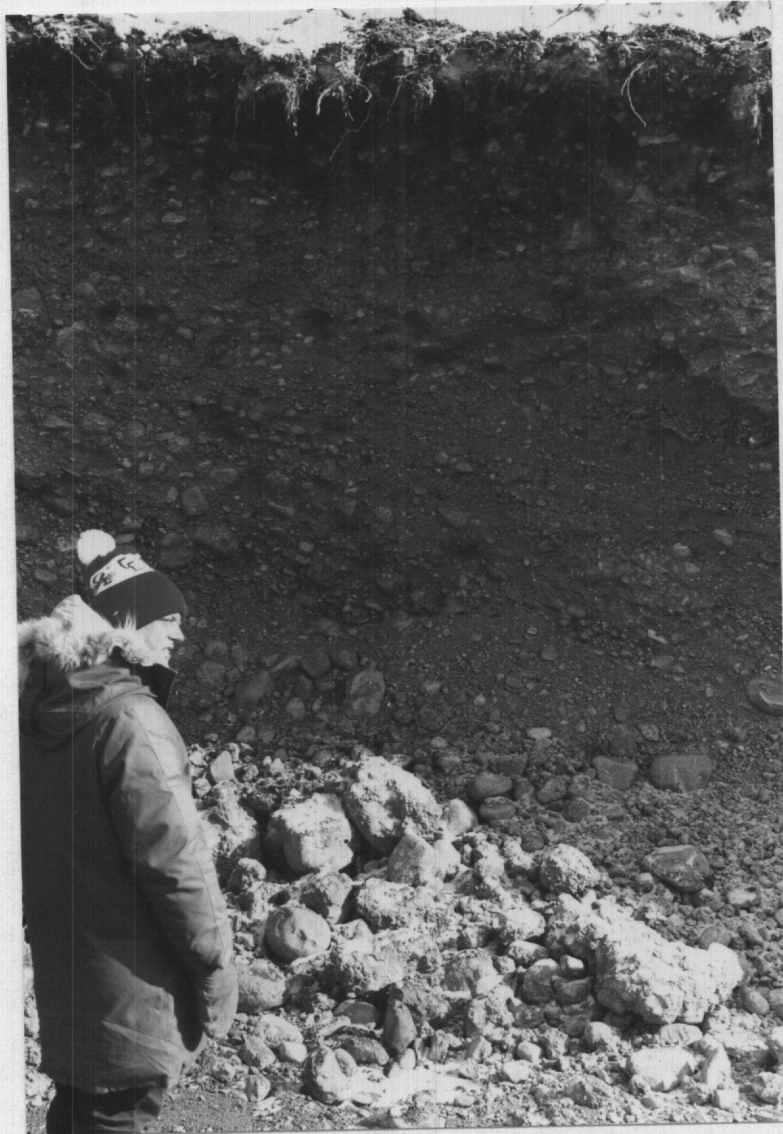
14. Deposit 5-6 (HR-109A): View of east end of newly developed pit, showing 3 m high face developed in cobbly moderately to poorly graded Class 3 material.
