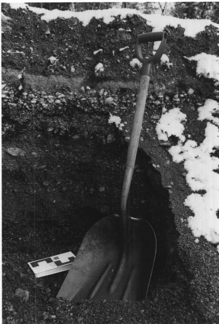
PHOTO 2: Foxhole South (Berton's) Pit, Deposit 5-69. In situ gravelly sand exposed at east end of existing pit.
