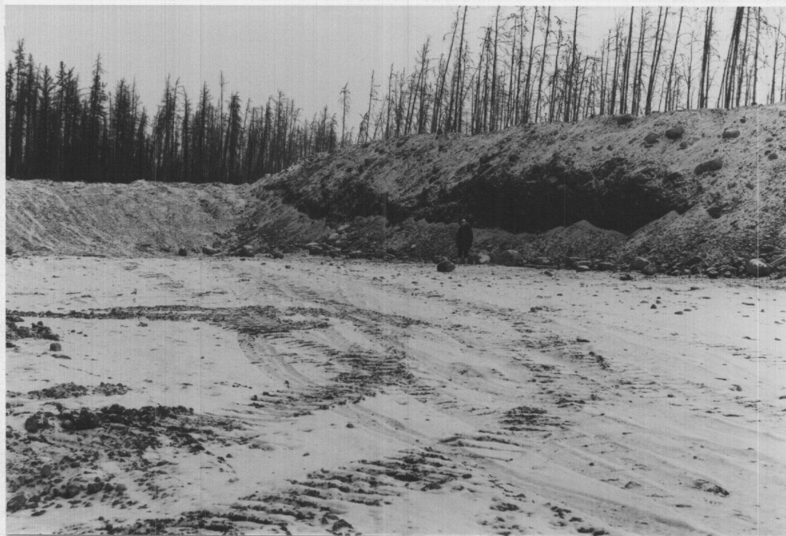
19. Deposit 5-14 (HR-124A): northeast corner of recently developed pit. 2.5 m to 3 m of gravel has been removed down to the underlying clay till.
