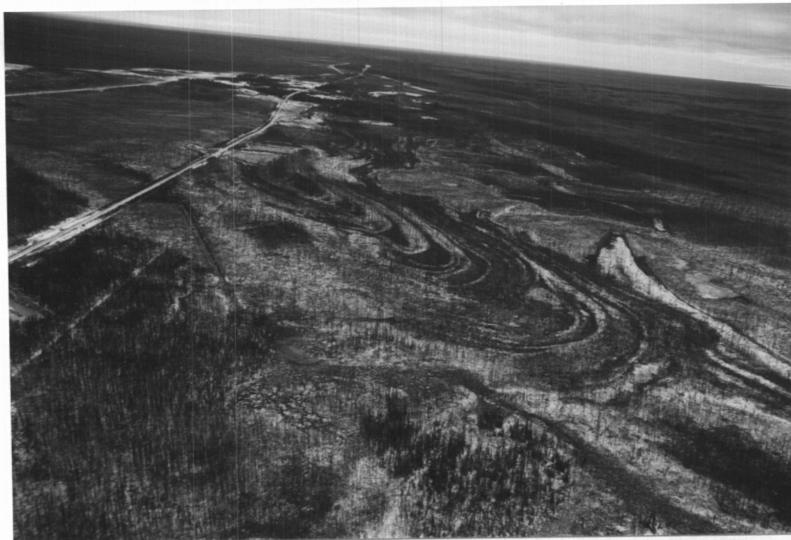
PHOTO 30: View to east along axis of Deposit 5-19 (HR-119, 121 and 122; Mile 21). Note prominent beach ridges, and depleted areas adjacent to C.N.R.
