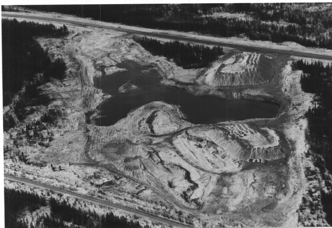
PHOTO 20: Deposit 1-15 (DPW km 66.6) is the source of limestone bedrock for crushing and blending with sand from Deposit 1-16.
