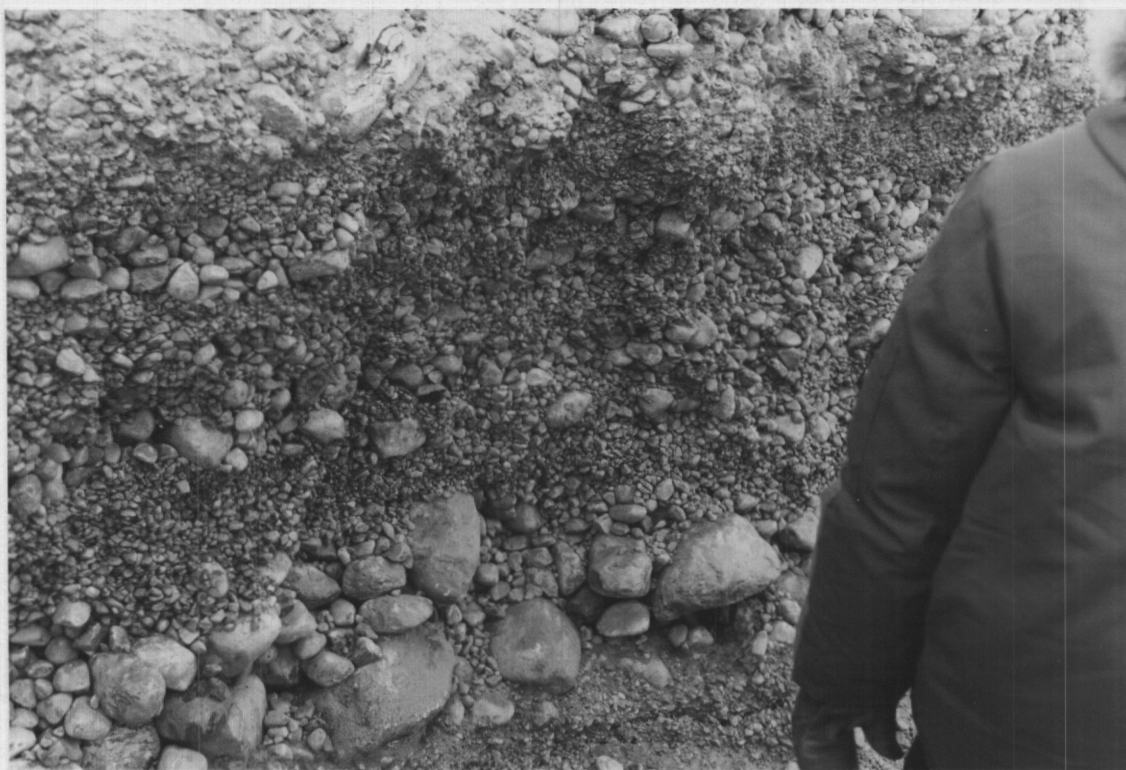
28. Deposit 5-40 (km 64.5): poorly and gap graded material in northern part of existing pit.
