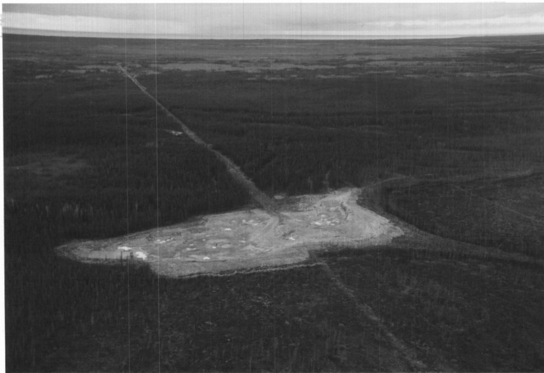
PHOTO 29: Deposit 5-14 (HR-124A), showing pit opened in winter 1986-1987 by DPW. The glacial till that underlies the granular aggregate is visible (as blue area) on pit floor to left.
