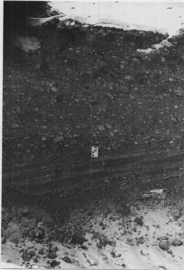
13. Deposit 5-6 (HR-109A): Close-up of east end of new pit, showing poorly-graded nearsurface aggregate overlying well graded fine sandy gravel.
