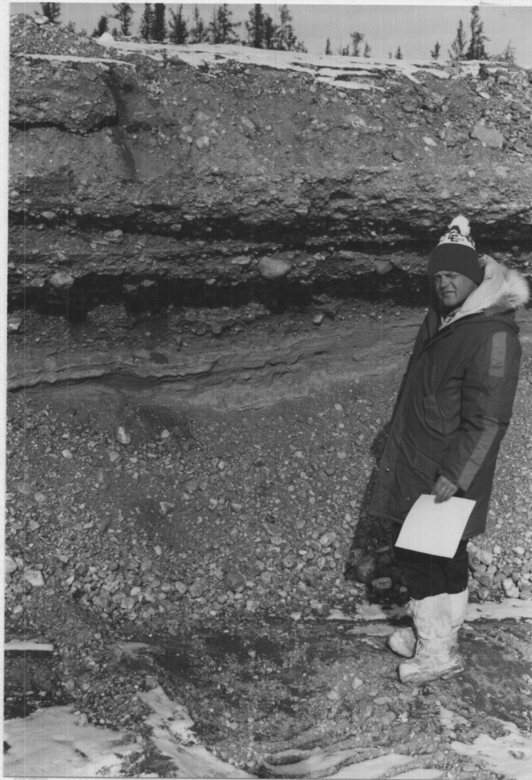
16. Deposit 5-6 (HR-109A): Close-up of "Pope's" pit, adjacent to winter road alignment and developed in well graded fine gravel.
