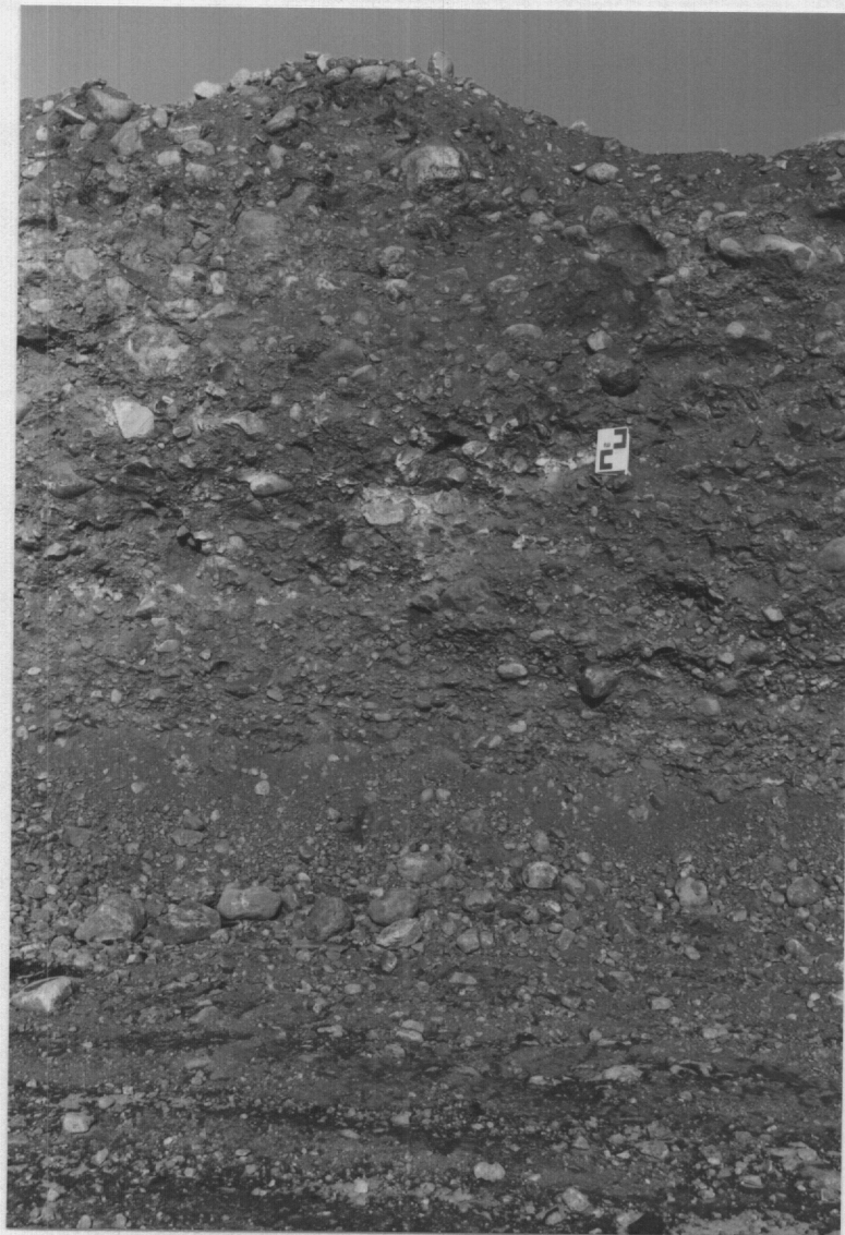
12. Deposit 5-6 (HR-109A): Close-up of poorly-graded and cobbly near-surface material exposed along north side of new pit at east end of deposit.
