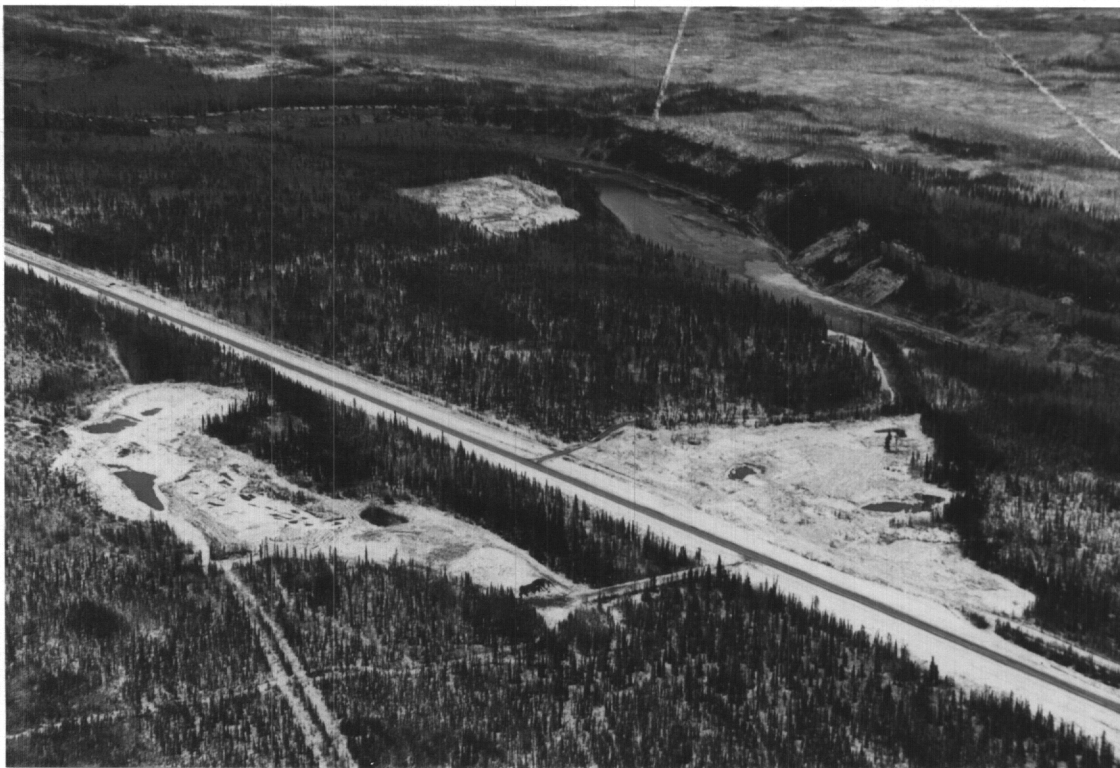
PHOTO 19: Deposit 1-16 (DPW km 77.2). Sand from this source is being blended, on an experimental basis, with crushed limestone from Deposit 1-15, to produce aggregate for highways maintenance.
