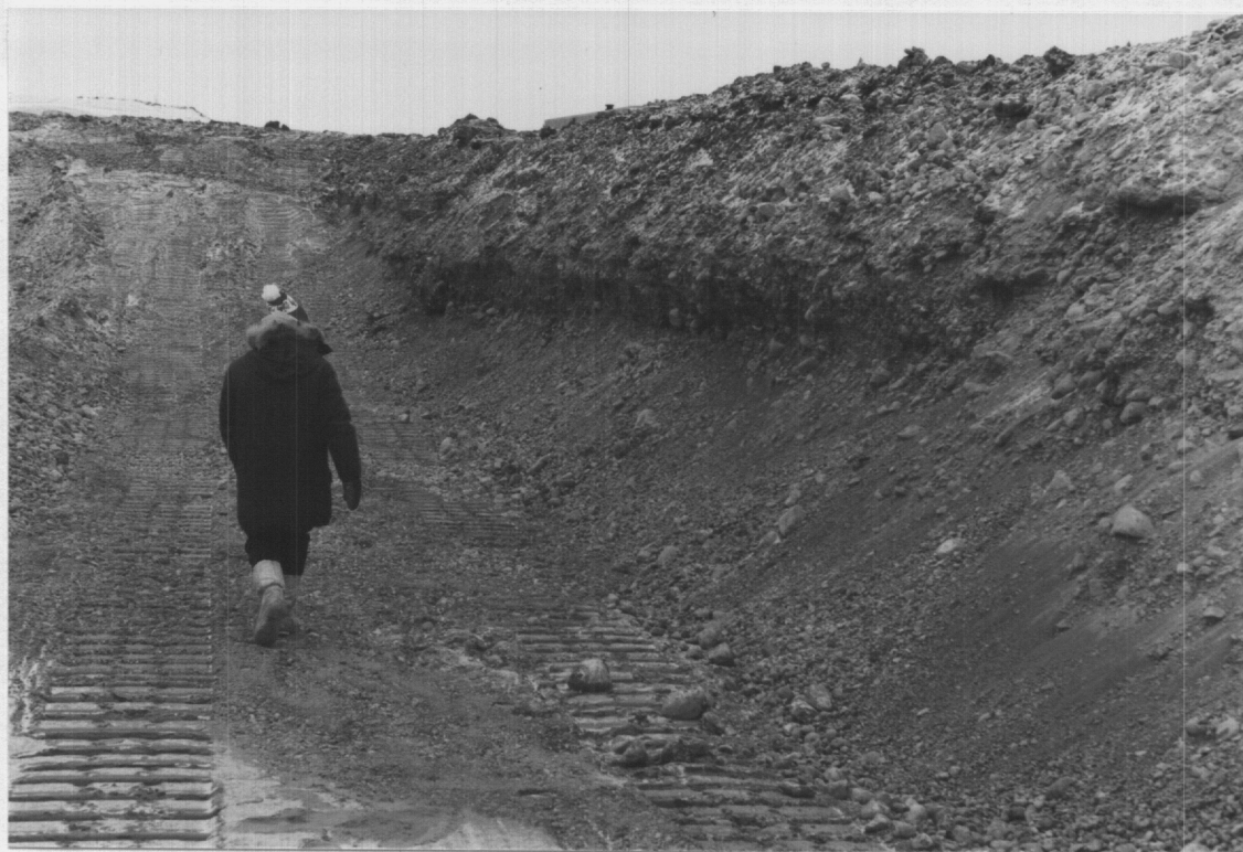
27. Deposit 5-40 (km 64.5): North end of existing pit, showing moderately to poorly graded aggregate, and uniform fine sand exposed in floor of pit.
