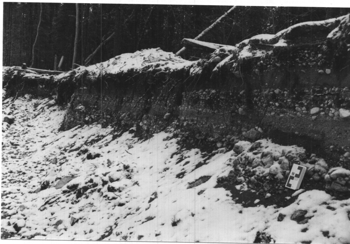
PHOTO 7: Salt Mountain North Pit, Deposit 5-69. Aggregate of variable composition and up to 2 m thick is exposed along northeast wall of pit.
