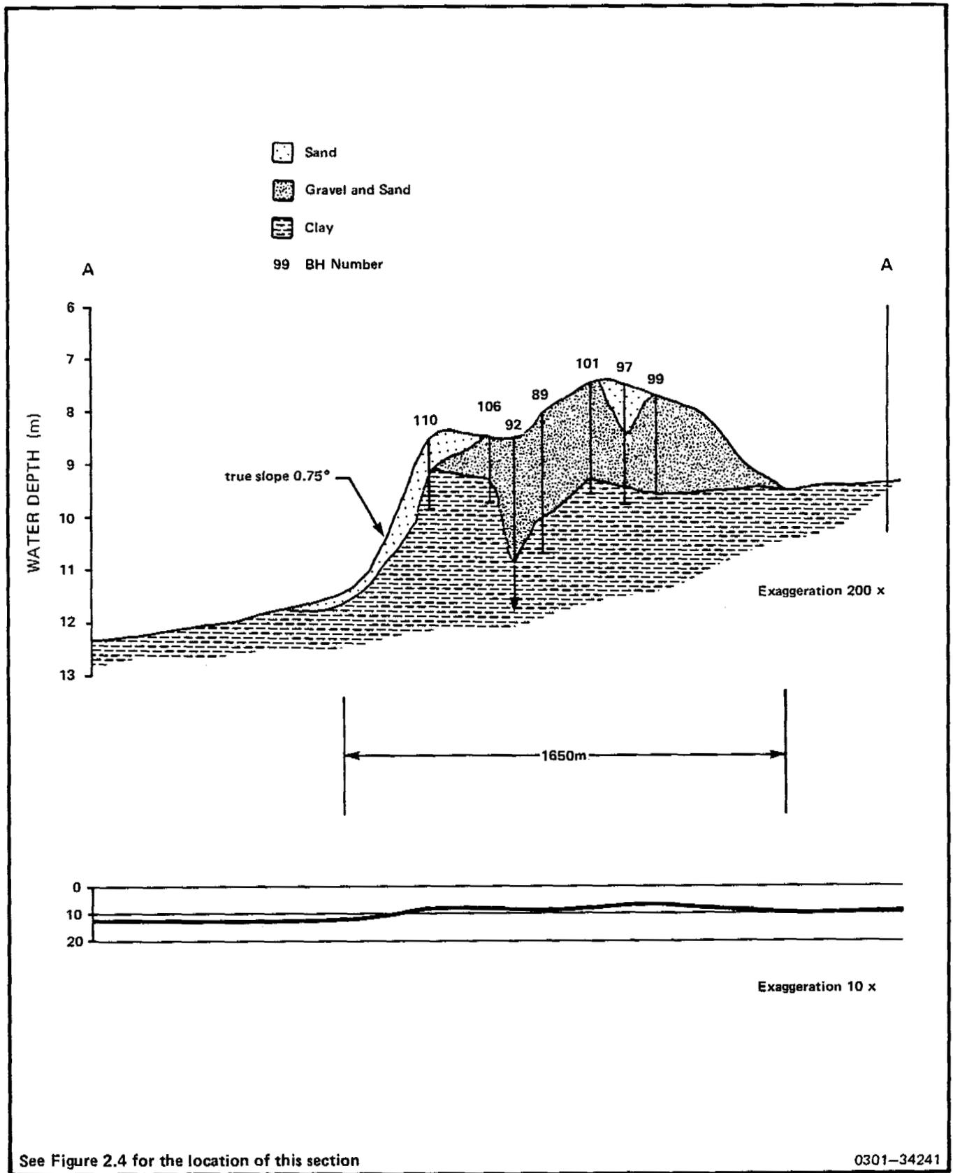
FIGURE 3.2 SECTION A-A THROUGH ISSIGAK DEPOSIT
