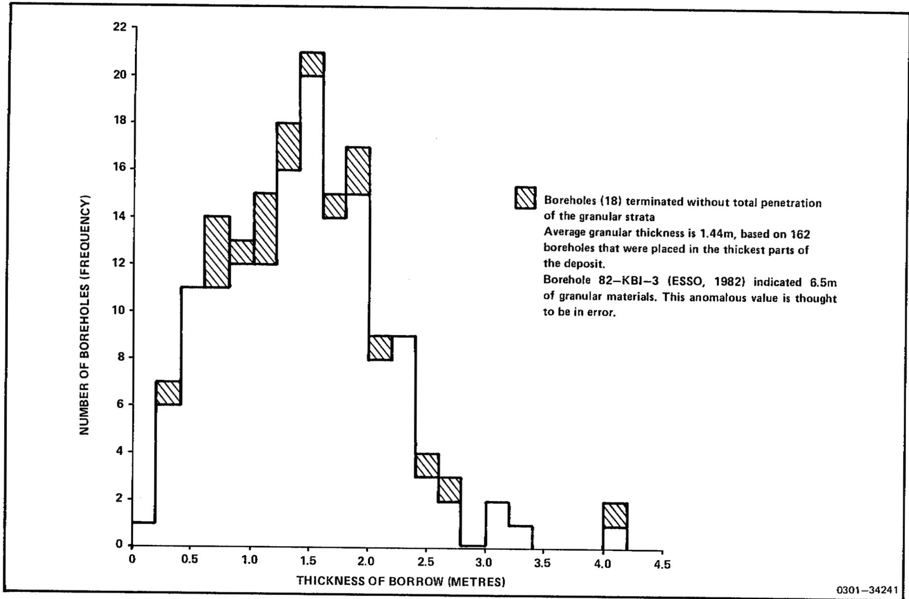
FIGURE 3.3 BORROW THICKNESS FREQUENCY PLOT FROM BOREHOLE DATA
