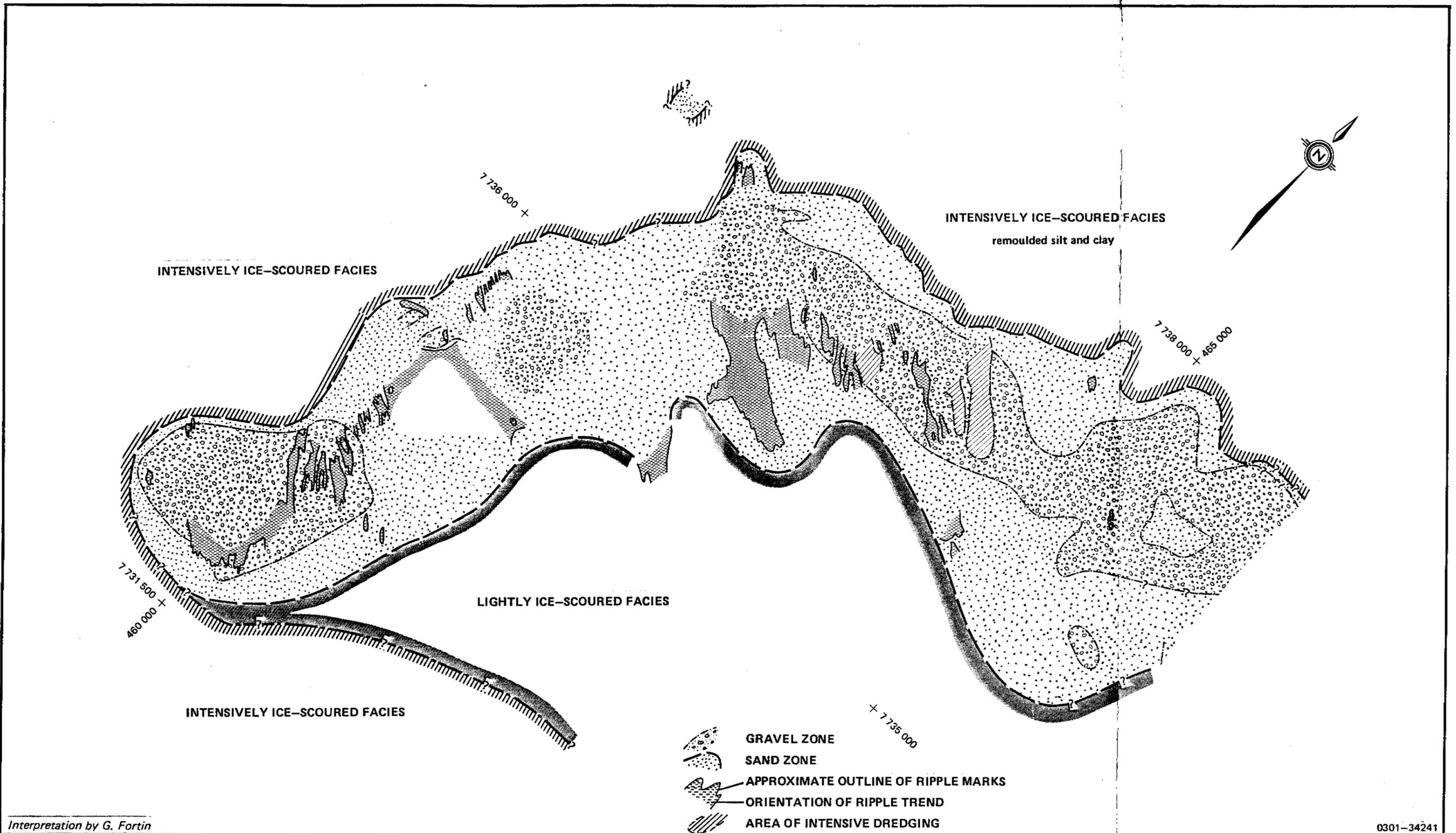
FIGURE 4.8 SIDESCAN INTERPRETATION OF SEABED CONDITIONS
