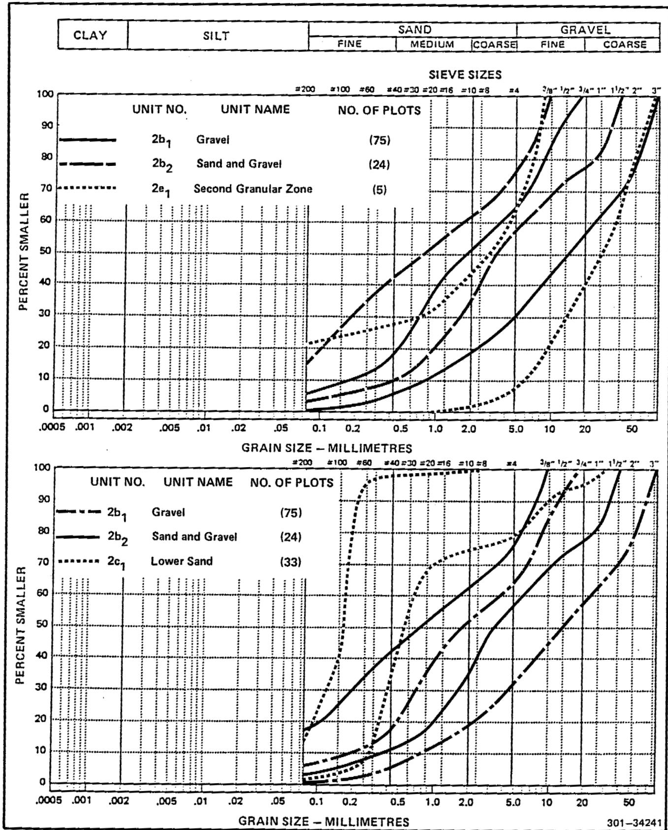
**FIGURE 4.2 GRADATION ENVELOPES FOR GRANULAR UNITS**
