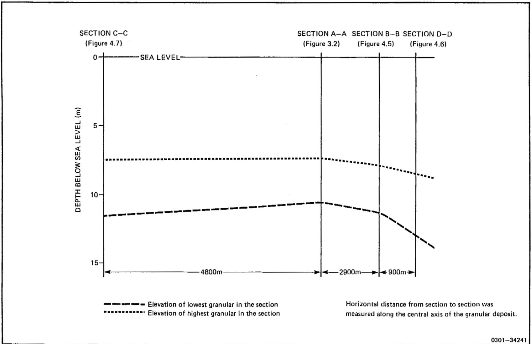
FIGURE 4.12    SOUTHWEST TO NORTHEAST SLOPE OF THE ISSIGAK DEPOSIT
