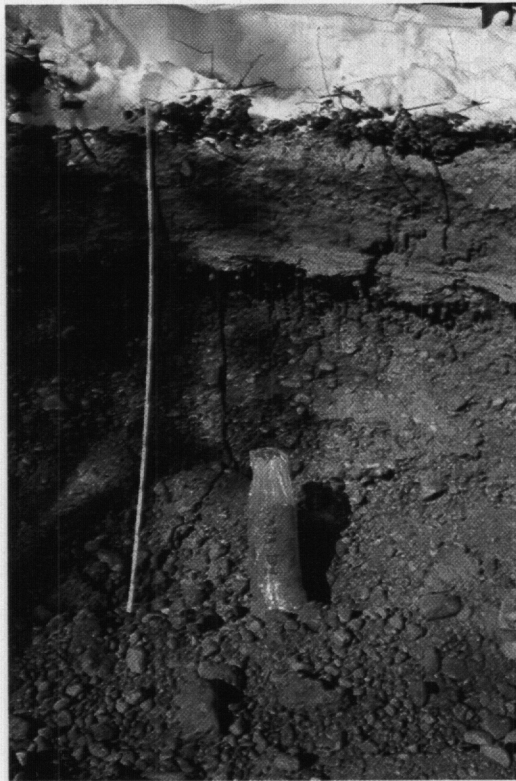
Photo 15: Test pit - sample at 3' level - 373-BT-1.
