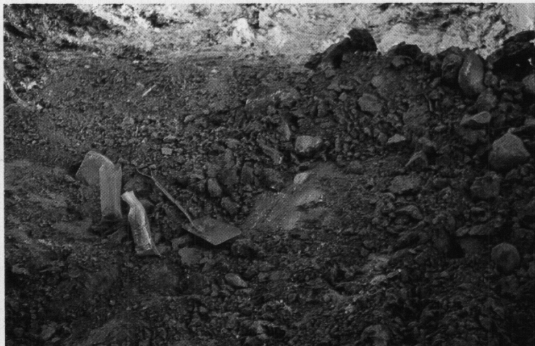
Photo 16: Test pit - sample at 4' level - 400-BT-1.
