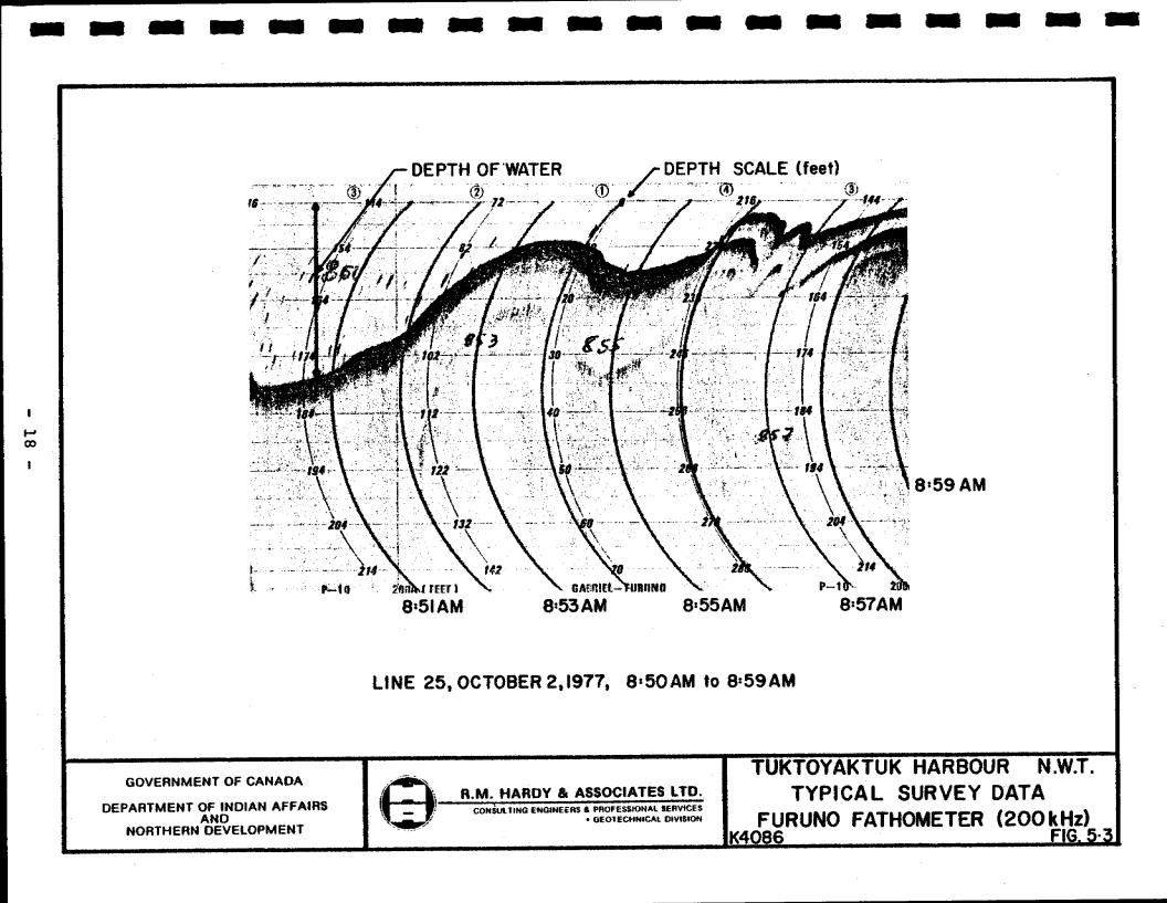
very little energy penetrates into the subbottom sediments, so that no further stratification can be distinguished. On the other hand, a soft bottom will only reflect part of the energy (e.g., in the order of 50%). The remaining energy will penetrate and sufficient energy is reflected from subsequent layers to allow recognition.
