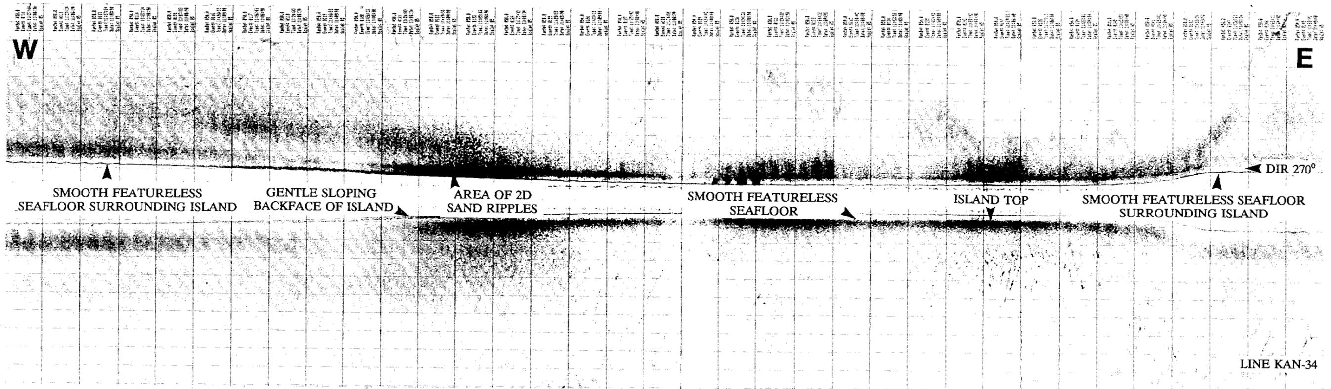
Figure 5.4.2 Sidescan data (Line KAN 34) displaying seafloor features characteristic of the G-42 island and surrounding seafloor.
