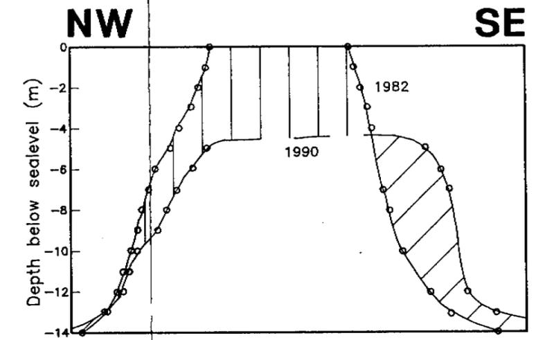
Conceptual Island Plan and Profiles Displaying Zones of Sediment Depletion and Accretion (top) and One Corresponding Island Example – Itiyok I-27 (bottom)
