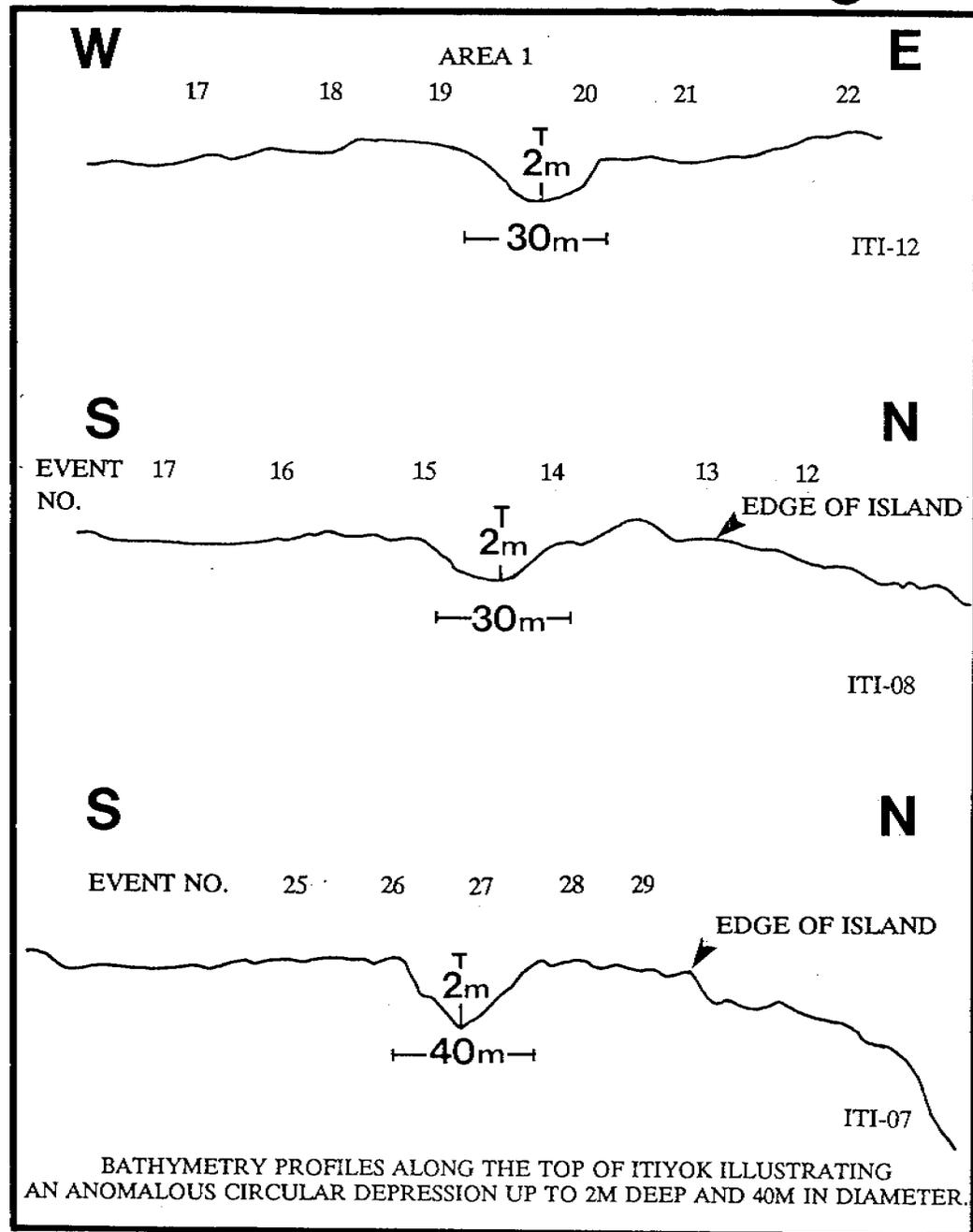
Figure 5.9.3 1990 site bathymetry map and 1990 echosounder records (Lines ITI 07, ITI 08 and ITI 12) displaying an anomalous depression on the northeast edge of the Itiyok island.
