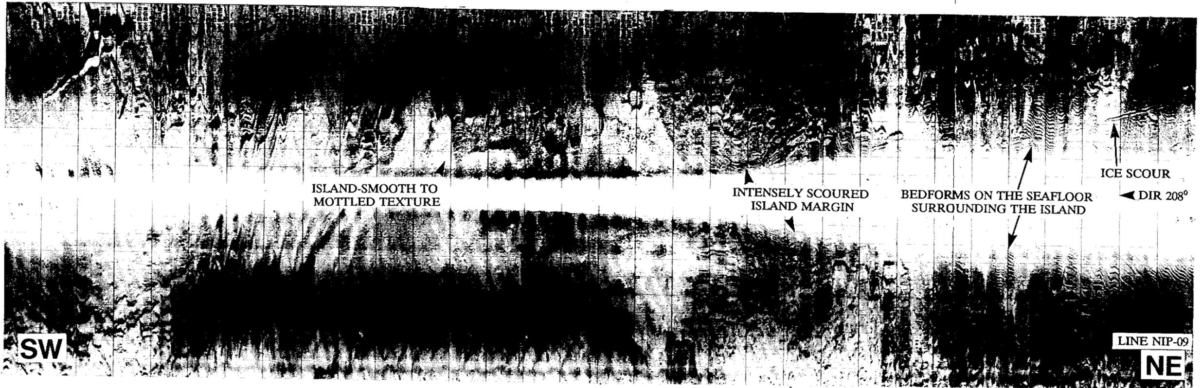
Figure 5.10.2 Sidescan data (Lines NIP 08 and NIP 09) displaying seafloor features characteristic of the L-19 island and surrounding seafloor.
