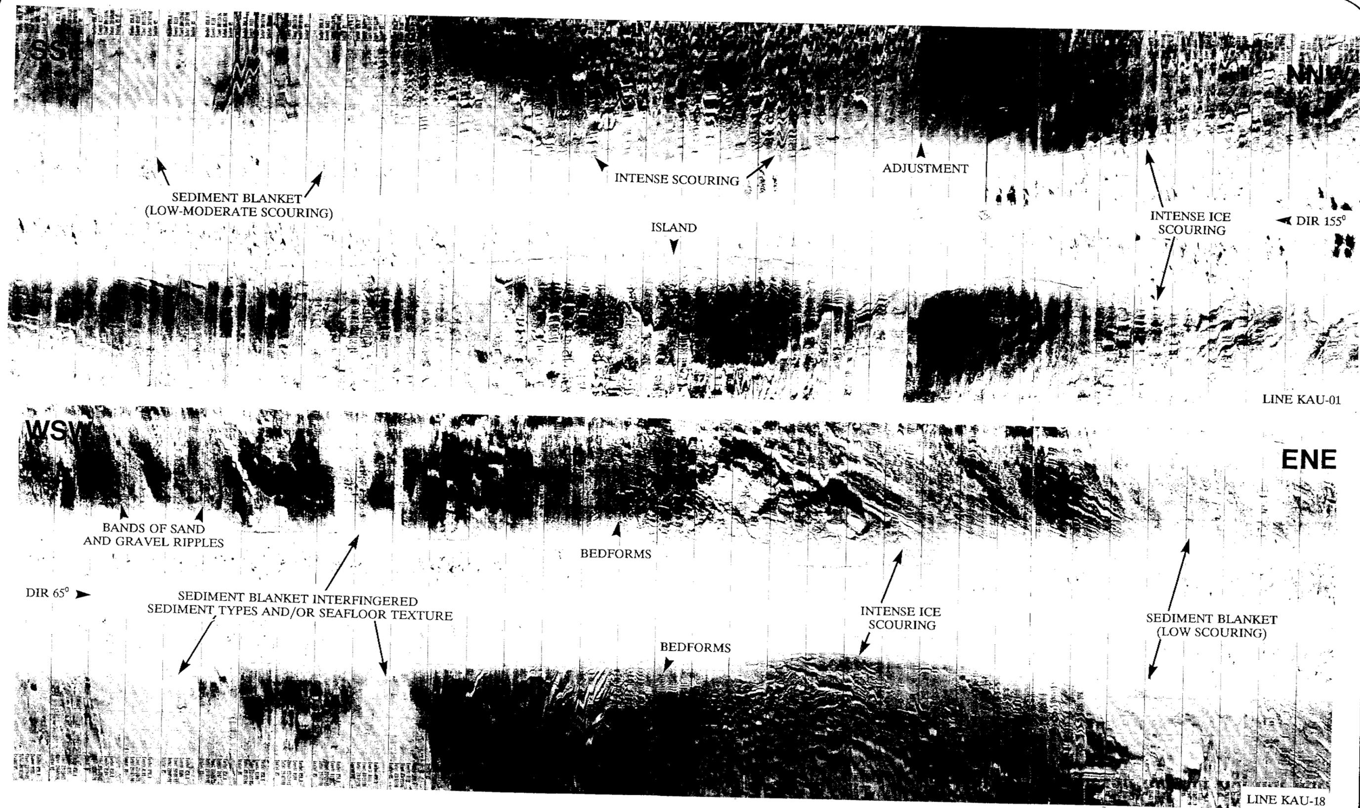
Figure 5.13.2 Sidescan data (Lines KAU 01 and KAU 34) displaying seafloor features characteristic of the I-43 island and surrounding seafloor.
