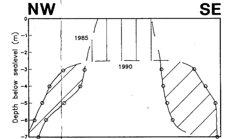
Conceptual Island Plan and Profiles Displaying Zones of Sediment Depletion and Accretion (top) and One Corresponding Island Example – Arnak K-06 (bottom)
