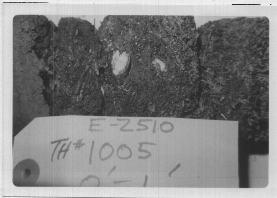
Photograph 34: A close-up of the sample shown in Photograph 33. The peat is category No. 15 using the Radforth system.
