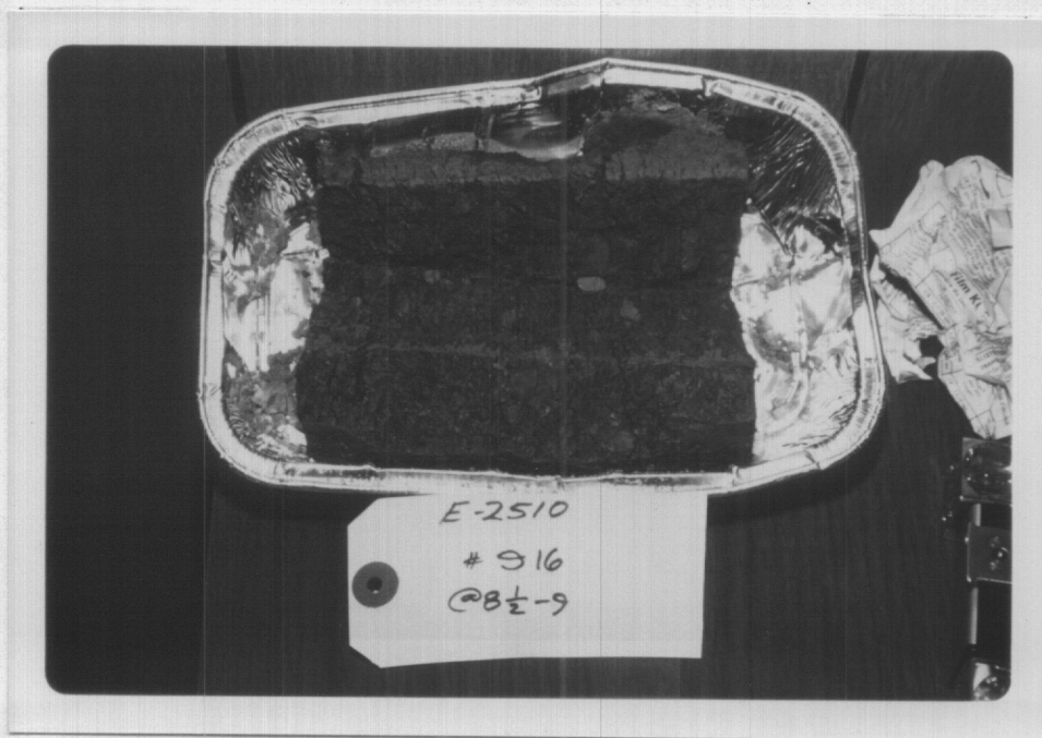
Photograph 30: A sample of silty-clay, medium plasticity, from Test Hole 916. Note the pebbles within this material. Water content was 25 percent.
