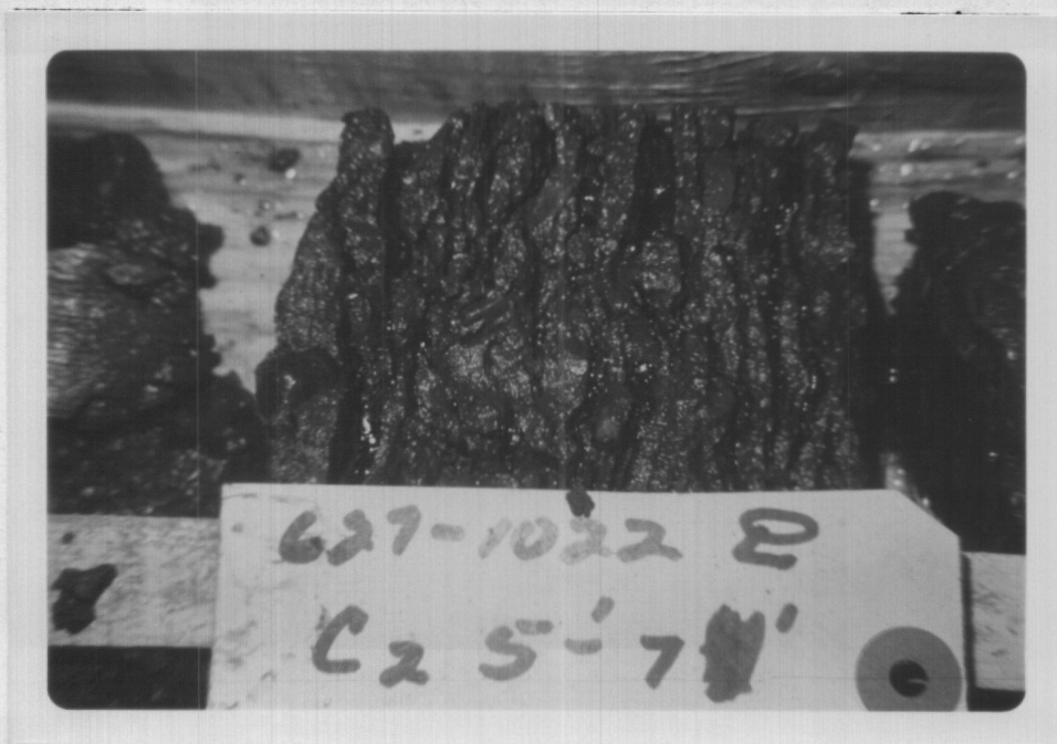
Photograph 35: A sample of clay from Test Hole 1022, depth interval 5 to 7 feet. This photograph was taken after the sample had started to thaw in the laboratory. The ice type and content was classified as Vs at 60 percent. The sample is lying on its side and the ice lenses would have been horizontal in the in situ position.
