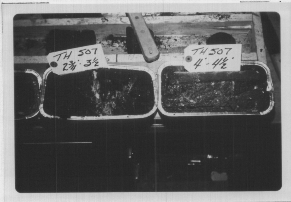
Photograph 20: Cores taken in Test Hole 507. On the left is a sample of organic clay with high ice content and on the right is a sample of clay till. In this case the clay till has a very high ice content.
