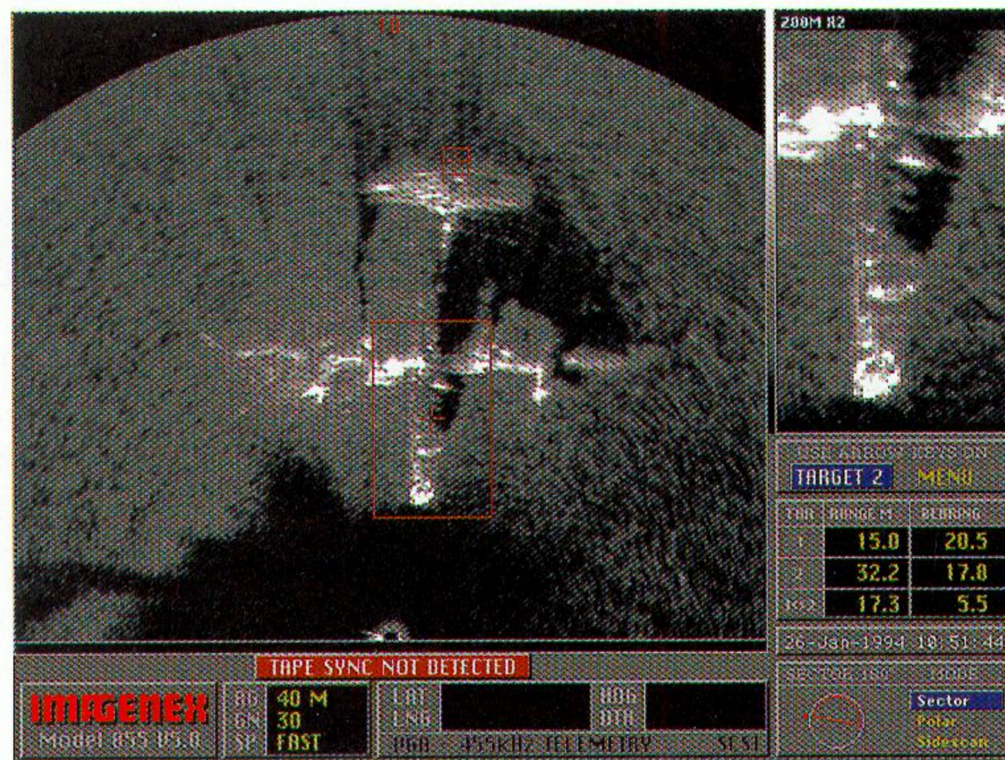
40 m sector scan, Convair PB4Y-2 Privateer, Lake Washington, Washington State, U.S.A., 675 khz.
