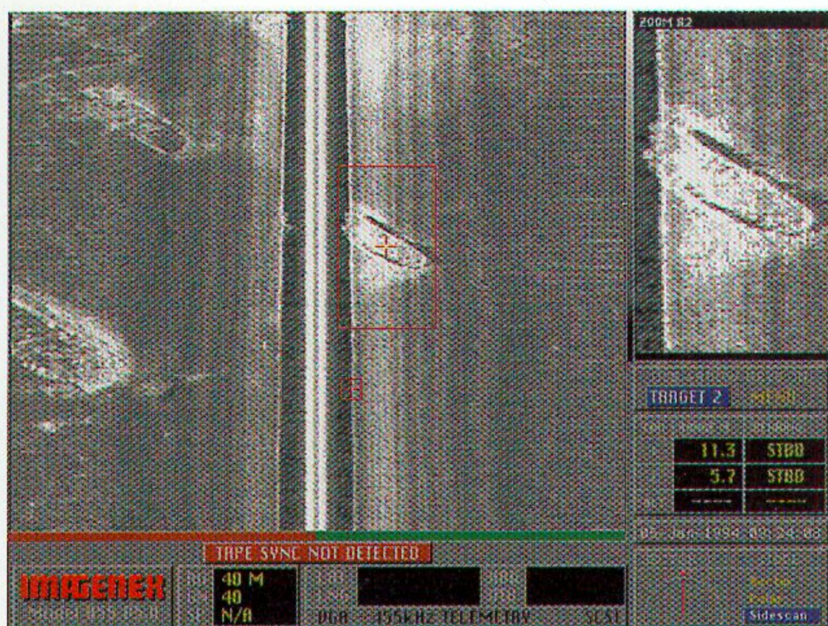
40 m side scan image showing 17th century wrecks in a Swedish harbor, 330 khz.
