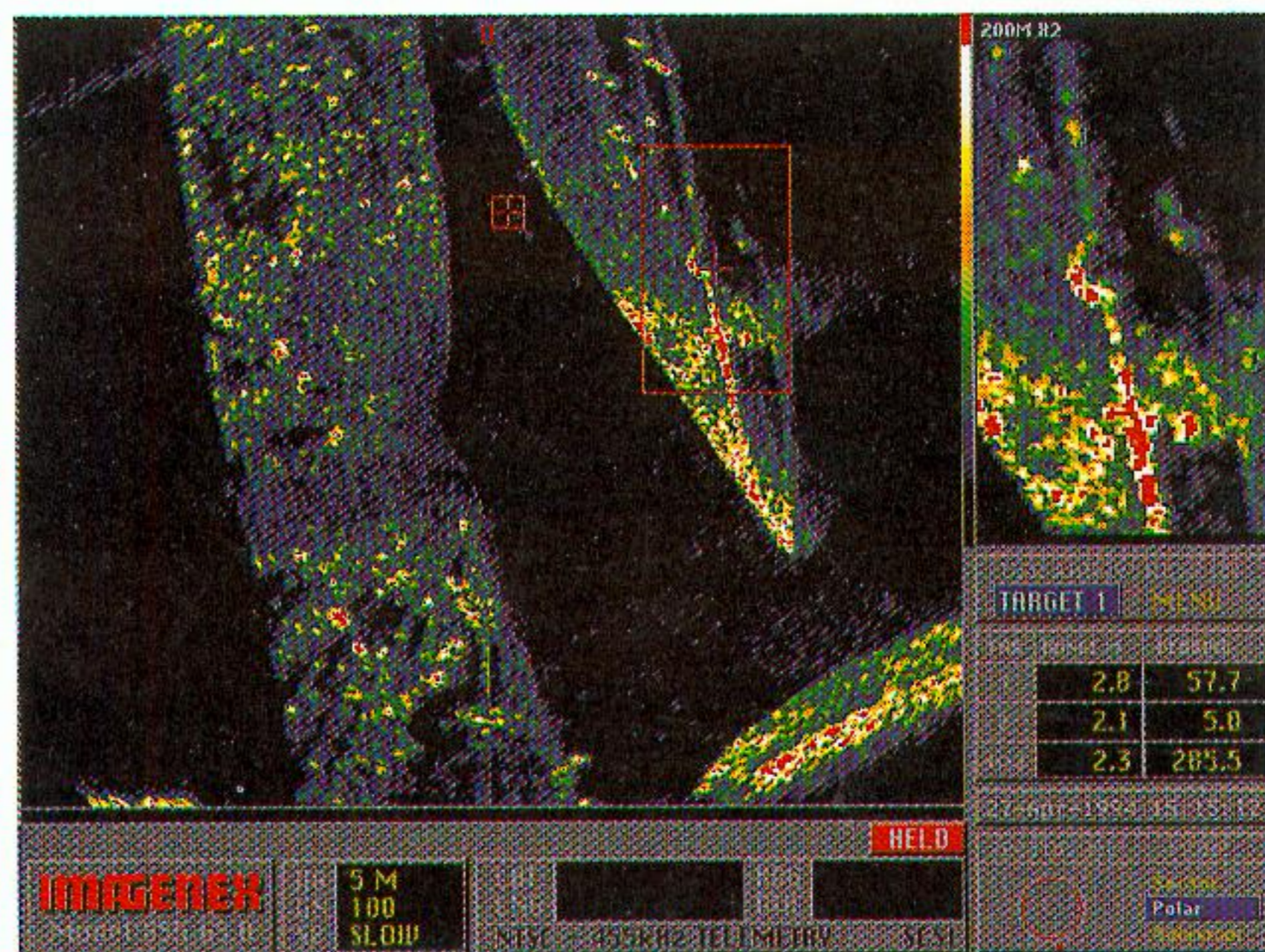
Ultra High Resolution sonar image. 5 m polar scan of the bow of a fishing boat and the bottom of a concrete floating dock. Sonar dome visible on fishing boat bow, 675 khz.
