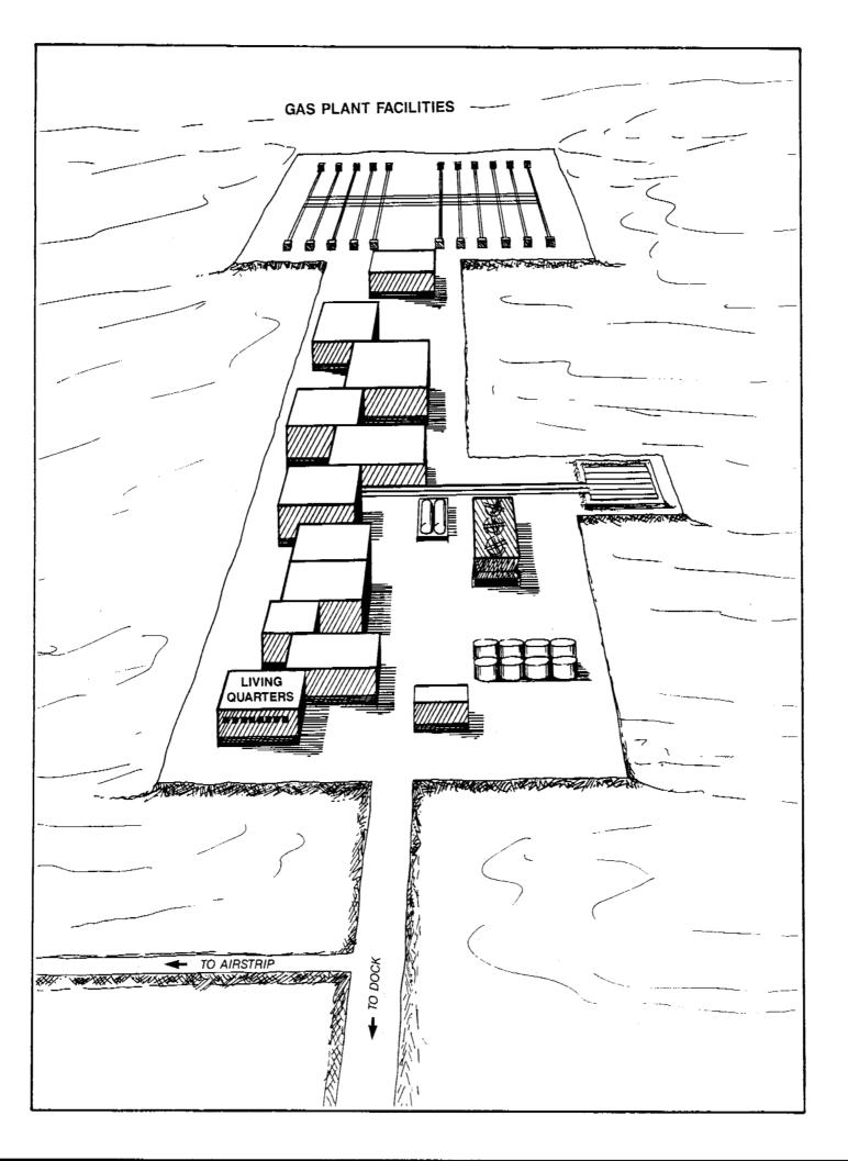
COMPRESSOR STATION - This artist's sketch shows a typical gas pipeline compressor station. Incoming and outgoing buried pipelines are indicated by the slightly disturbed ground surface in the foreground. Pig traps and valve assemblies are also shown in the foreground. Buildings housing compression and cooling equipment together with pipe storage racks appear in the centre of the sketch. Maintenance and warehouse building appear in the background.
