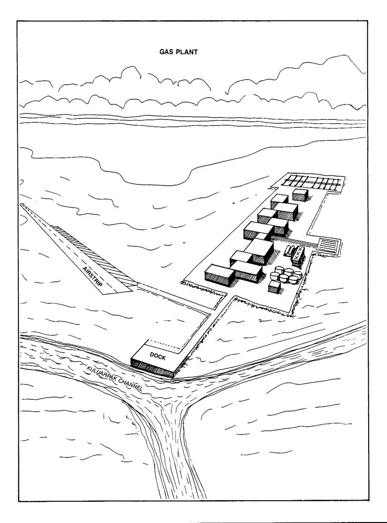
GAS PLANT FACILITIES - This sketch presents a closer view of the gas plant illustrated in the previous drawing. Buildings in the foreground would house staff and function as warehouses and maintenance workshops. Buildings in the middle of the sketch would house processing equipment. Aerial coolers, storage tanks and a ground flare are also shown and a well pad and production wells appear in the background. All of the facilities are situated on a gravel pad.
