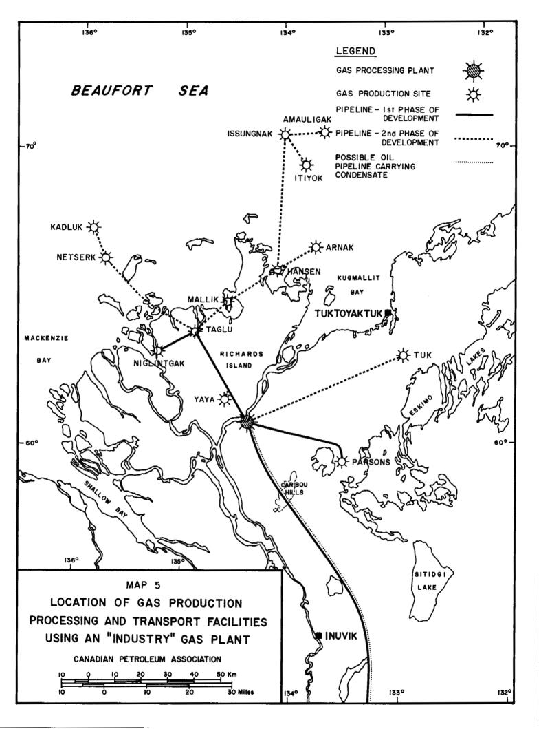
would be piped to the shared plant before processing. In later stages of development, other reserves, both onshore and offshore, would also be connected via gathering lines designed to carry unprocessed gas. Map 5 illustrates the likely location of gas development facilities within the planning region if an "industry" gas plant were utilized.
