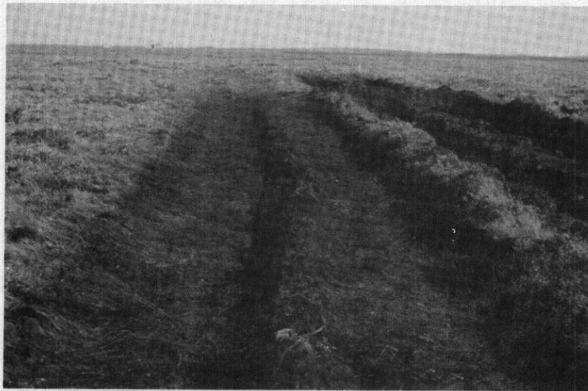
Fig. 13 Test Site 3, 60 Pass Heavy Load
