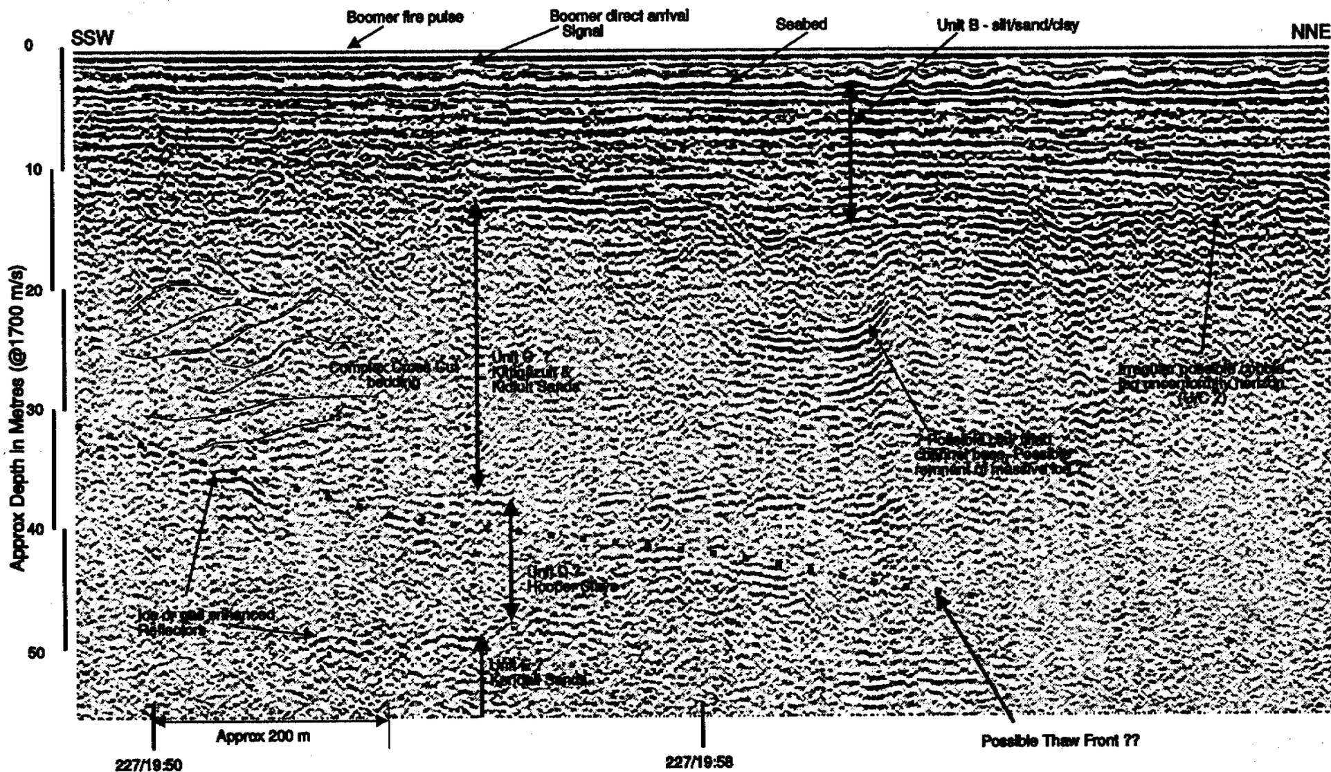
Figure 24: Boomer record from the inshore end of the Pipeline Corridor indicating the thick sequence of Recent materials infilling the collapse basin and the deeper seismostratigraphic sequences. Region offshore from this record is masked by shallow gas above, or cobble lag sediments at the unconformity surface.
