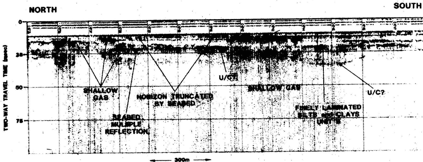
Boomer record from Line NAH-88-PIP1 in the inshore region near North Point showing reflecting horizons within unit B that are truncated at the seabed which implies recent seabed erosion and/or reworking of Unit B(?) materials in the shallow water regions.
