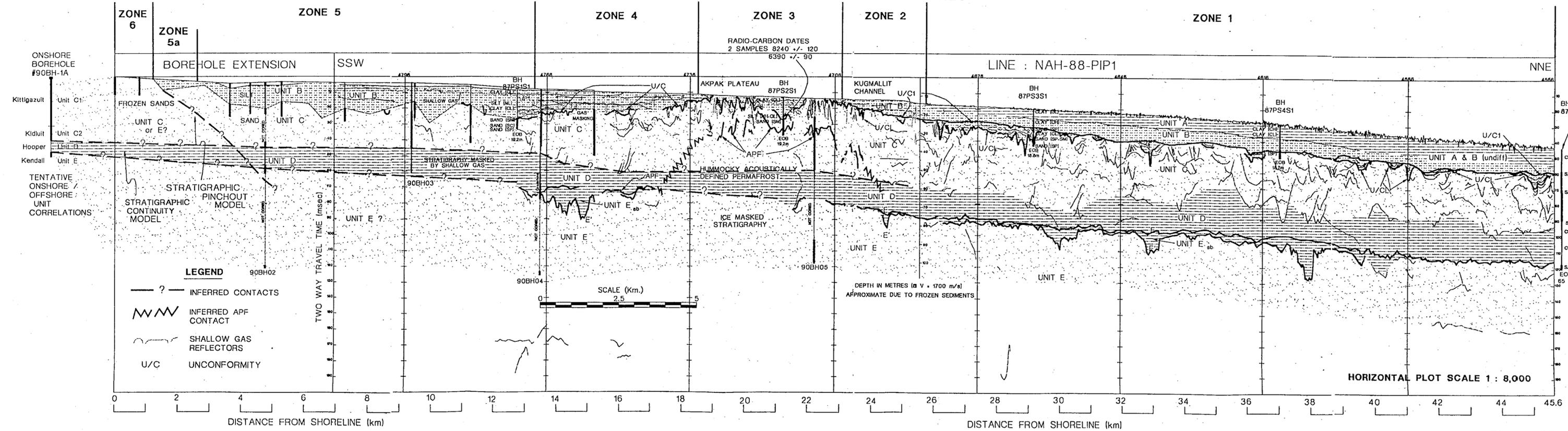
Line Drawing profile along centre of pipeline corridor based on boomer and airgun seismics with borehole extension into the nearshore shallow water zones.
