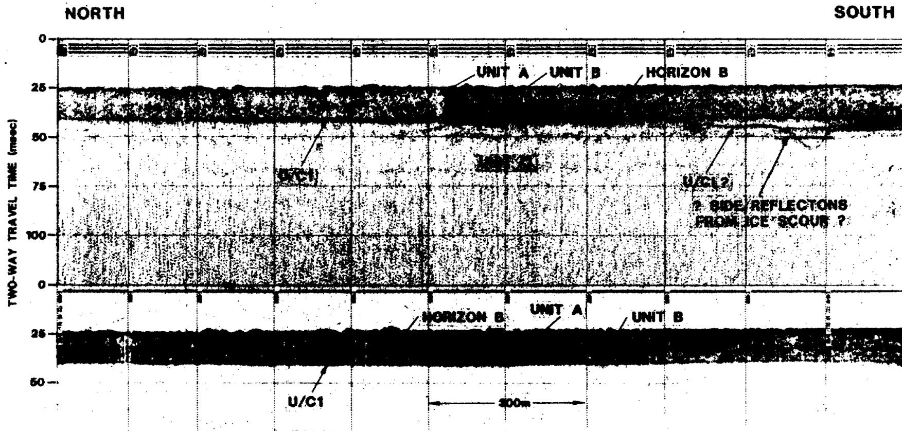
IKB Boomer and 7 kHz Profiler record from line NAH-88-PIP1 within the Kugmatt Channel area which displays an amorphous poorly delineated reflecting horizon within the surficial Holocene sediments that is tentatively identified as the top of Unit B.
