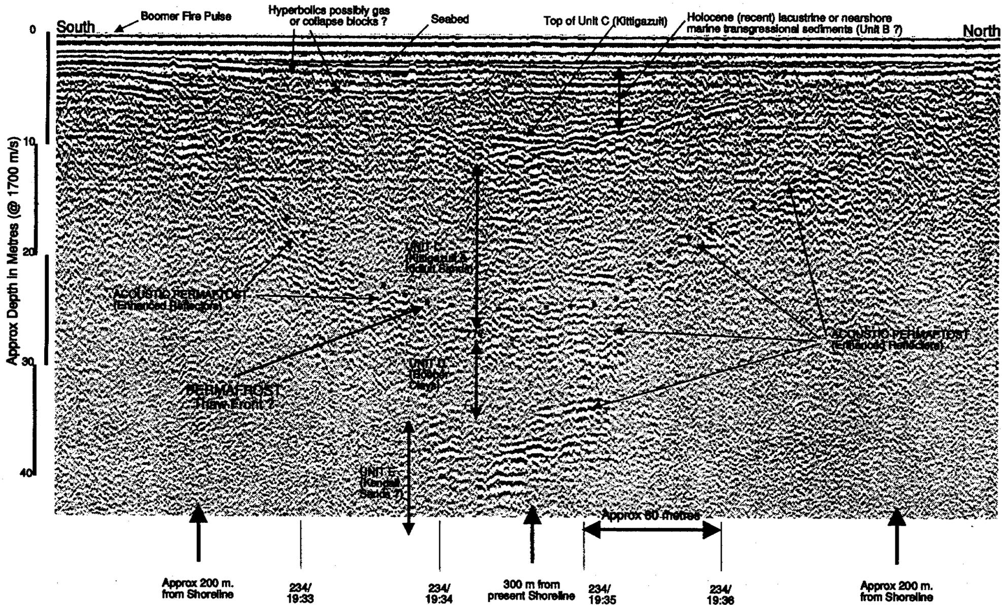
Figure 26: Boomer record paralleling the western shoreline of Hanson Harbour to the south of Reindeer Island. Line arcs slightly away from shore and shows APF reflectors rapidly dipping away from shore correlating with slight increase in the water depth.
