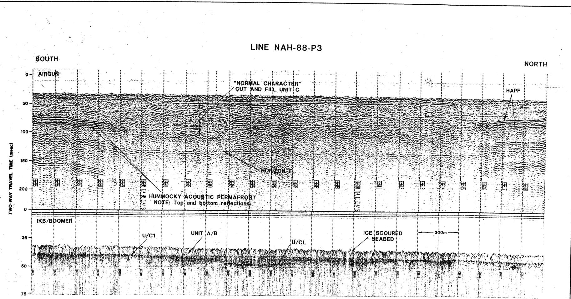
Airgun and Boomer profiles of Line NAH-88-P3 from the offshore region of Akpak Plateau displaying the complex cut and fill channelling patterns of acoustic reflectors within Unit C which defines its "normal character", along with double HAPF reflections and the dual unconformities on the top of Unit C.
