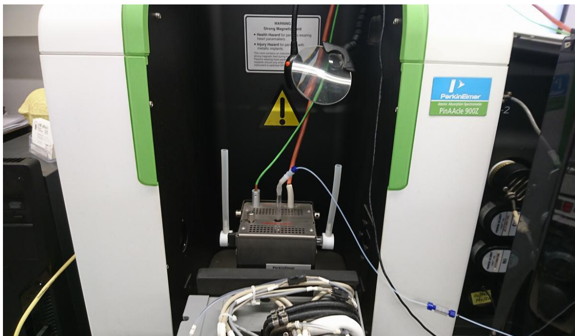
Photo 4. Perkin Elmer PinAAcle 900z™ atomic absorption spectrometer with quartz cell and heating mantle set up with Perkin Elmer FIAS – 100™ flow injection unit for CVAAS mercury analysis.
