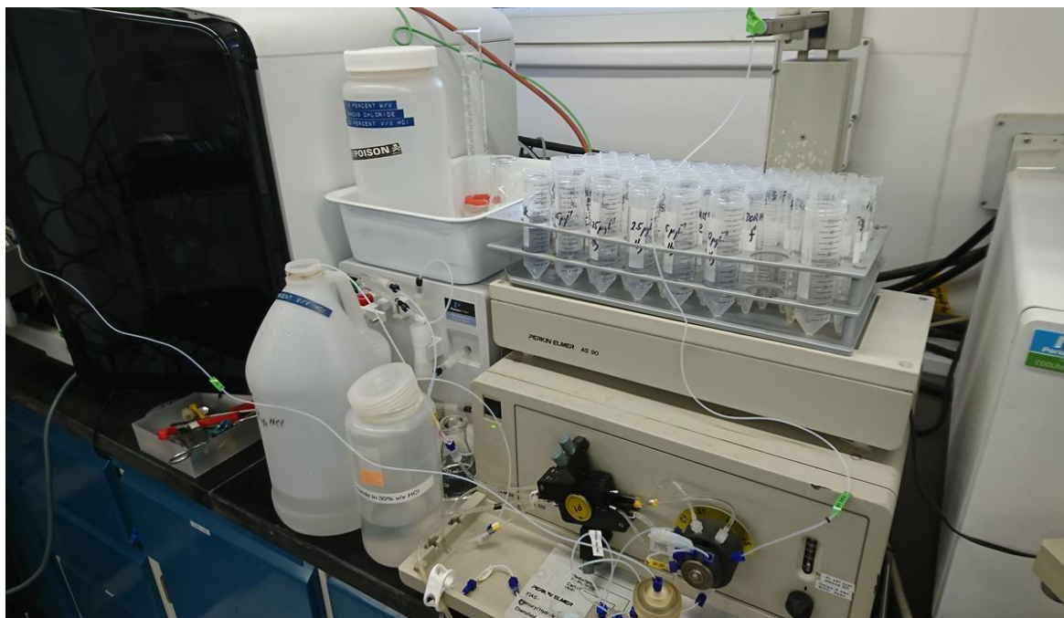
Photo 5. Perkin Elmer FIAS – 100™ flow injection unit with Perkin Elmer AS90™ autosampler set up for automated CVAAS mercury analysis.
