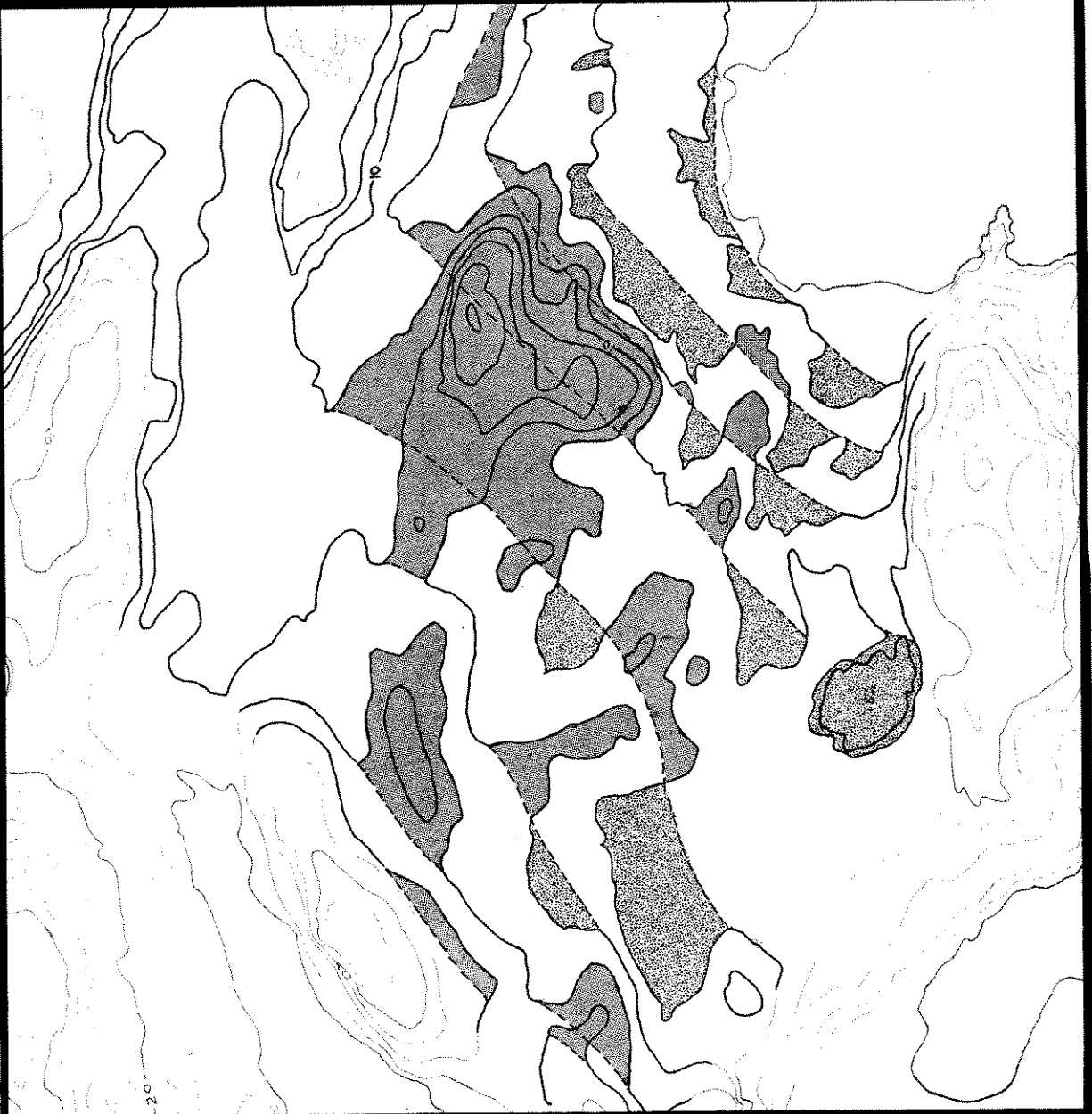
FIG. 6.1 CUT AND FILL OF THE VILLAGE AREA
