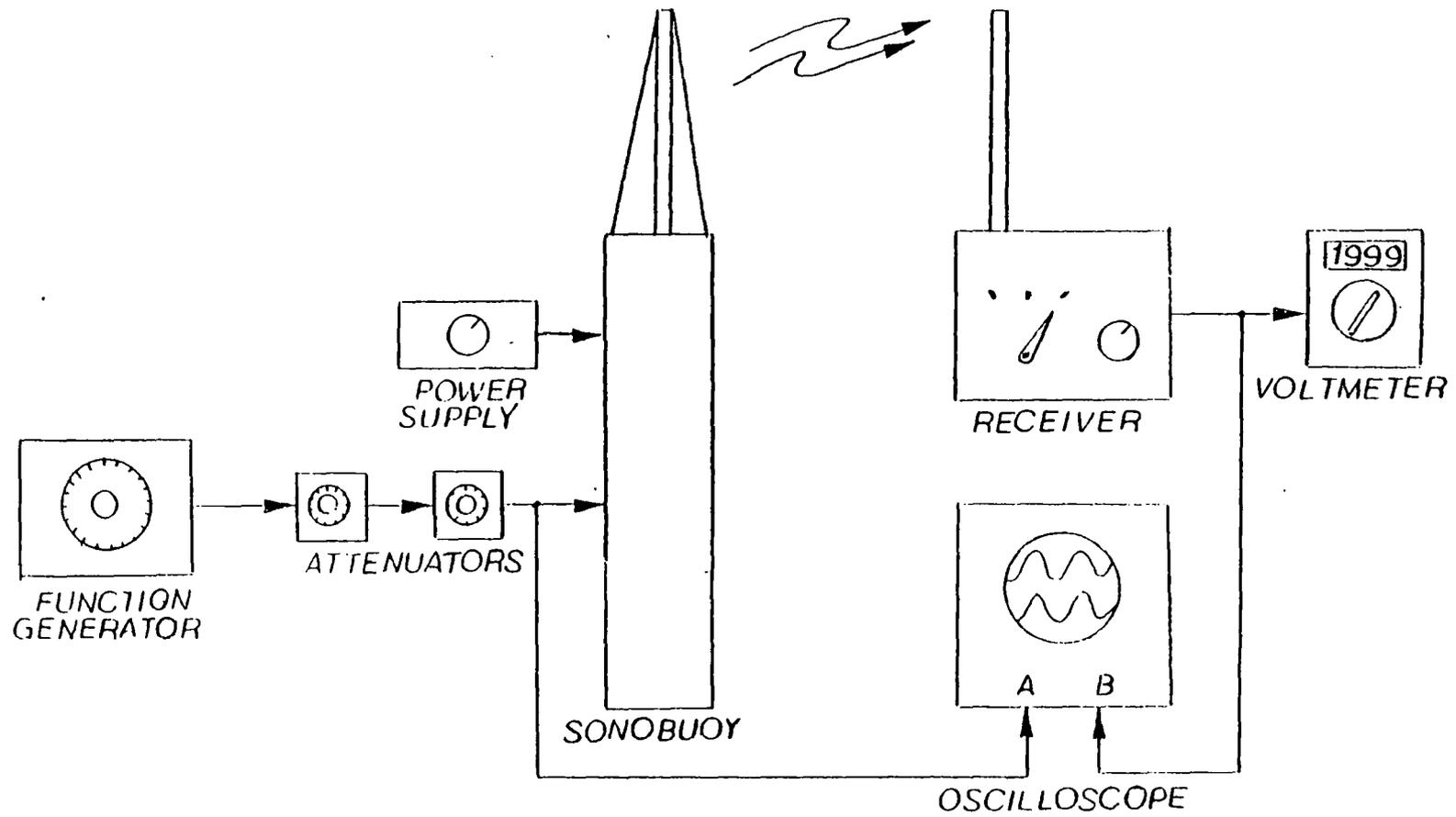
FIGURE 5. Electronic calibration test equipment
