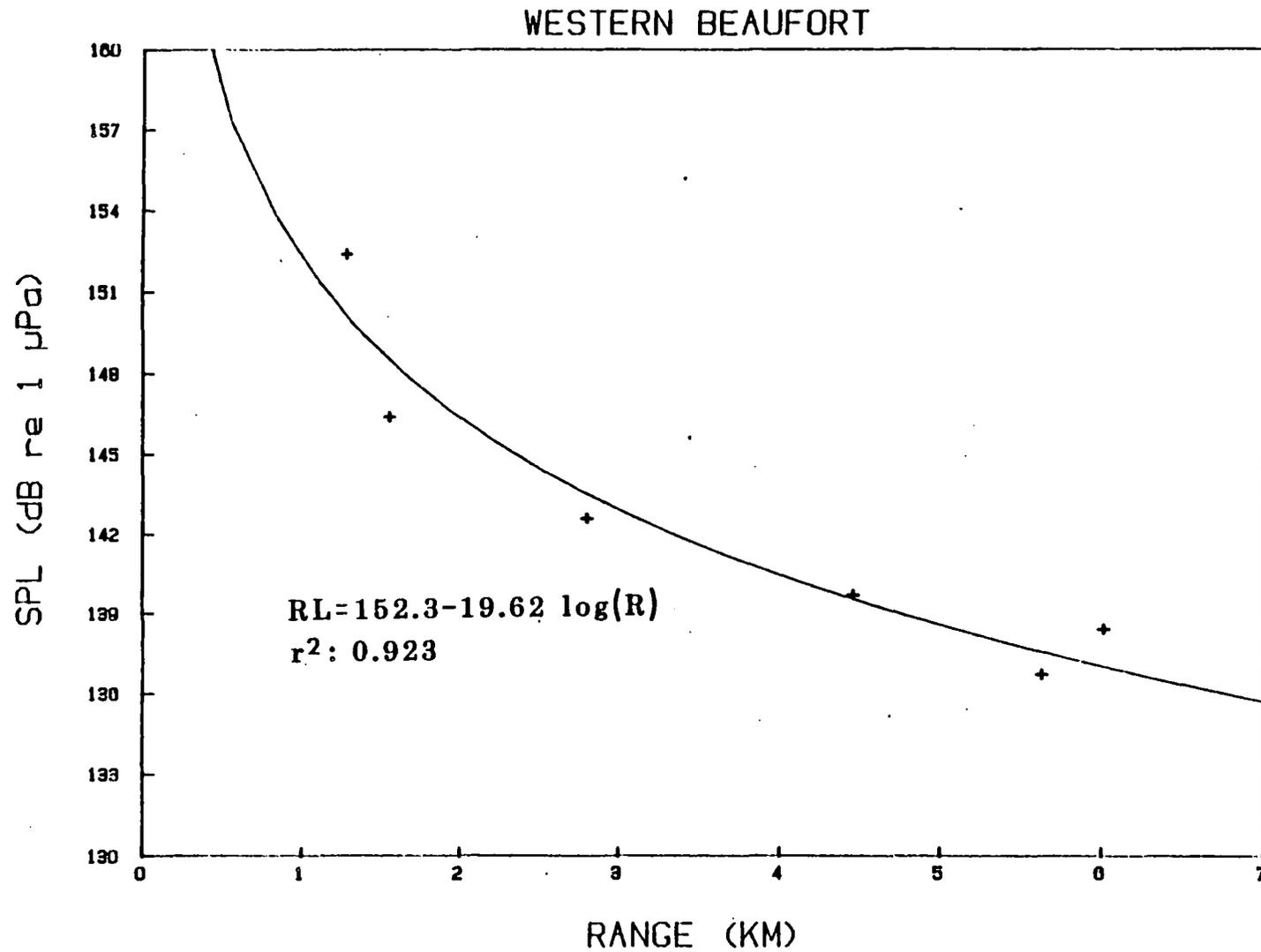
FIGURE 14. Western Beaufort seismic level vs. range (logarithmic curve fit: RL = receive level, R = range in kilometers,  $r^2$  = coefficient of determination).
