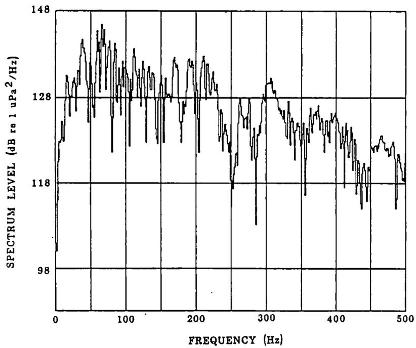
FIGURE 10. Western Polaris seismic pulse, 2.66 km range, time-domain (top) and frequency-domain (bottom)
