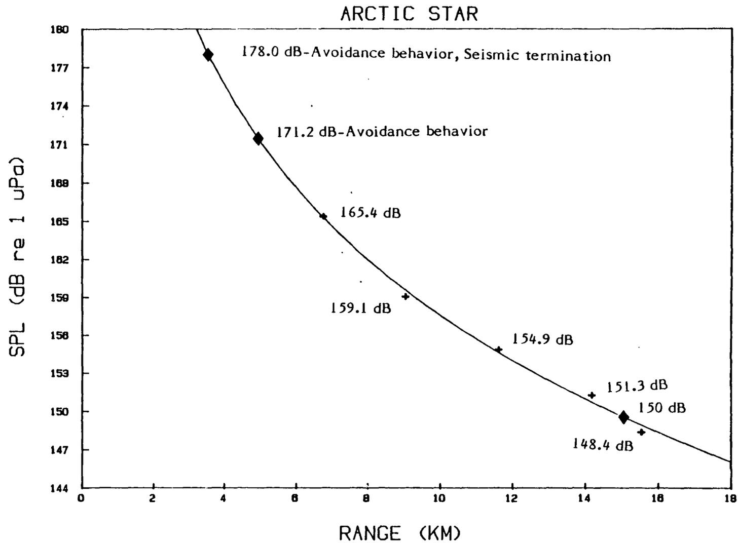
Figure 15. Received seismic sound levels versus range for the Arctic Star. Line is a least squares regression line to fit to the measured sound levels. ◆ = Estimated sound level; + = Measured sound level.
