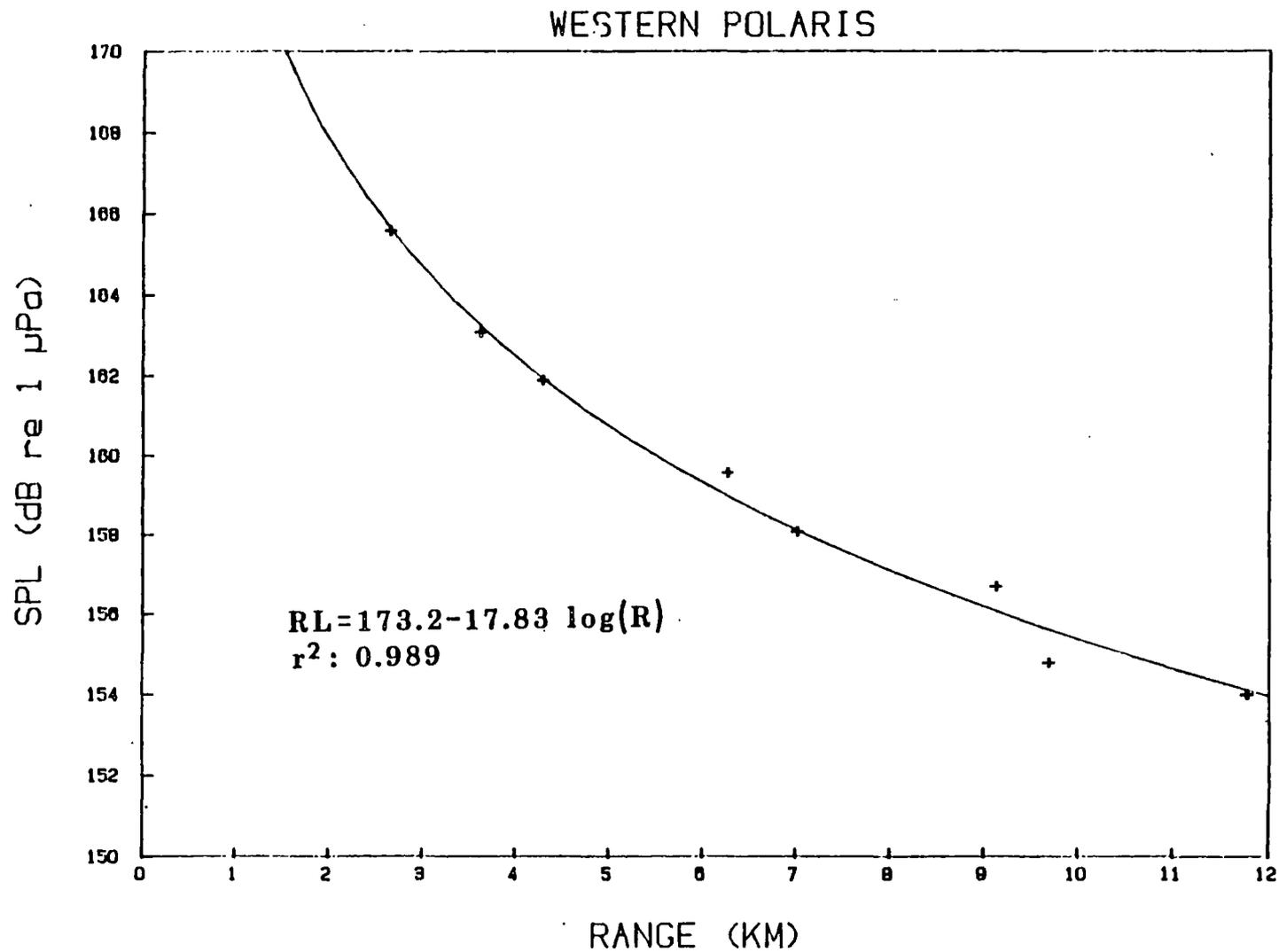
FIGURE 17. Western Polaris seismic level vs. range (logarithmic curve fit: RL = receive level, R = range in kilometers,  $r^2$  = coefficient of determination).
