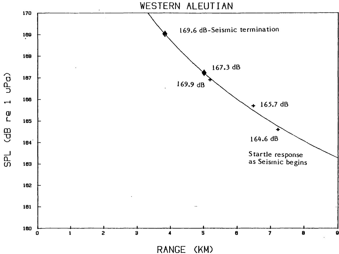
Figure 12. Received seismic sound levels versus range for the Western Aleutian. Line is a least squares regression line fit to the measured sound levels. ◆ = Estimated sound level; + = Measured sound level.
