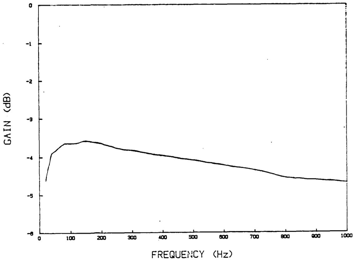
FIGURE 4. Modified 41A sonobuoy frequency response, 0-300 Hz (top), 0-1000 Hz (bottom)
