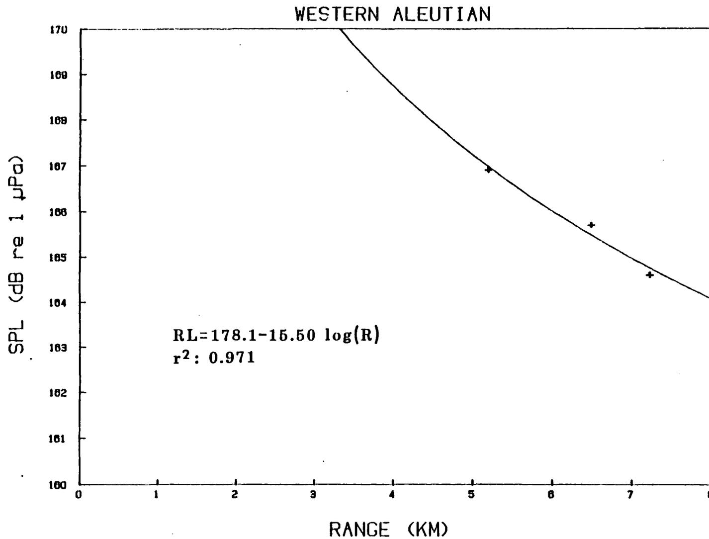
FIGURE 16. Western Aleutian seismic level vs. range (logarithmic curve fit: RL = receive level, R = range in kilometers,  $r^2$  = coefficient of determination).
