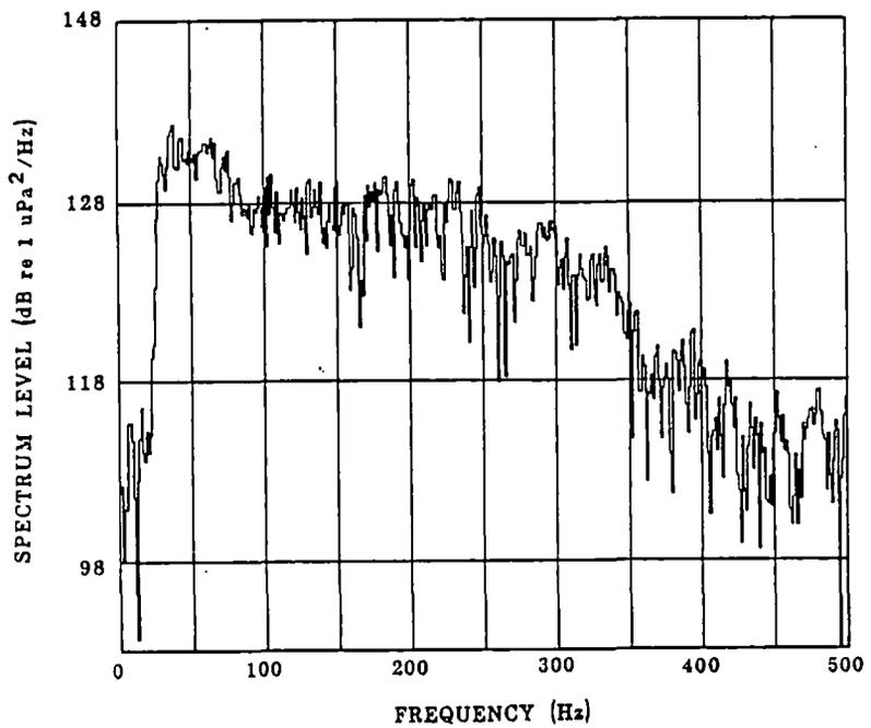
FIGURE 11. Western Aleutian seismic pulse, 5.84 km range, time-domain (top) and frequency-domain (bottom)
