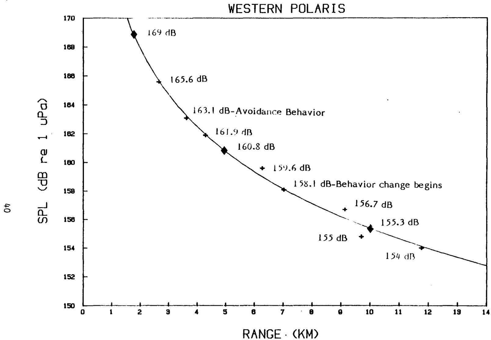
Figure 18. Received seismic sound levels versus range for the Western Polaris. Line is a least squares regression line fit to the measured sound levels. ◆ = Estimated sound level; + = Measured sound level.
