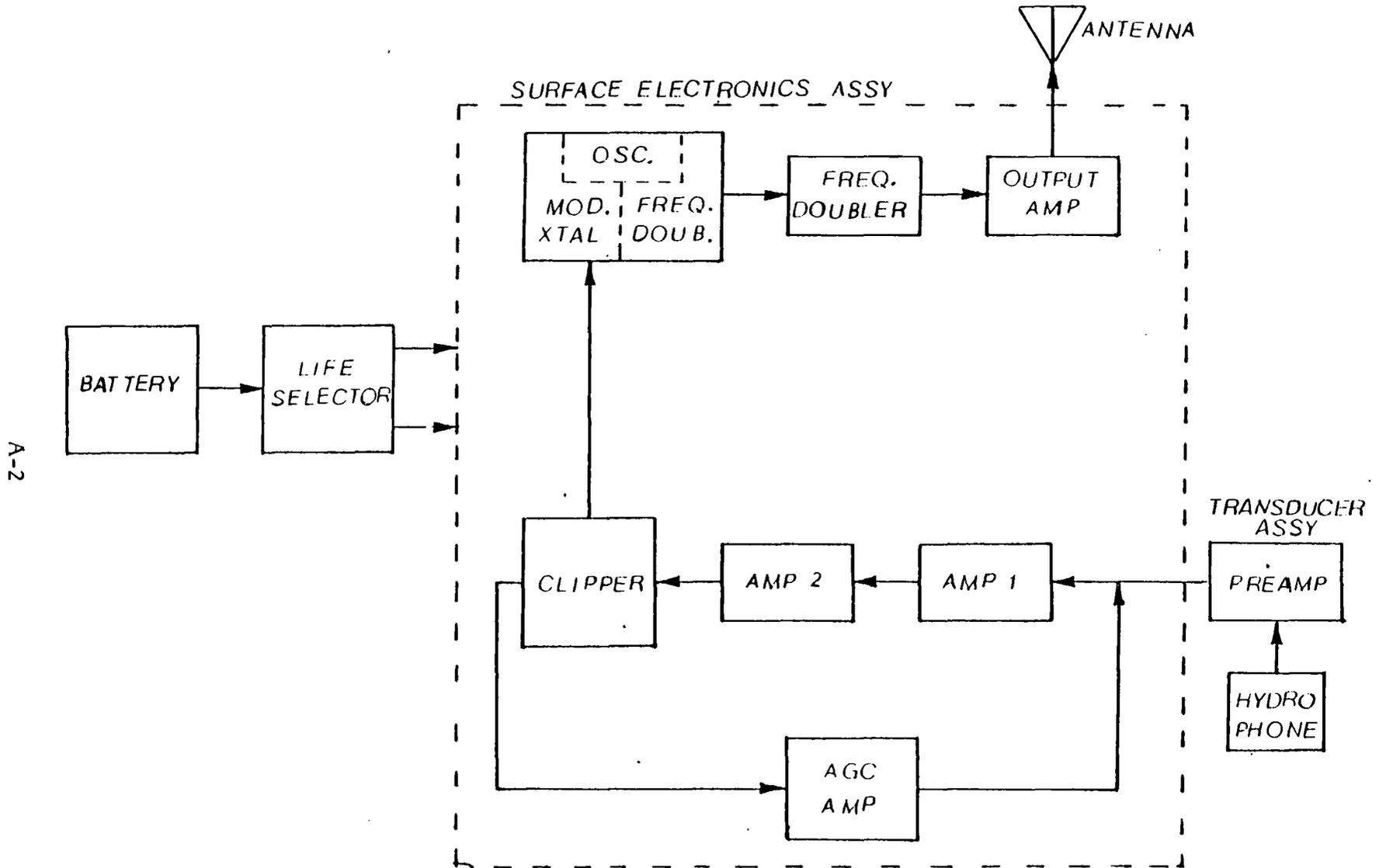
FIGURE 1. Unmodified 41A sonobuoy functional block diagram
