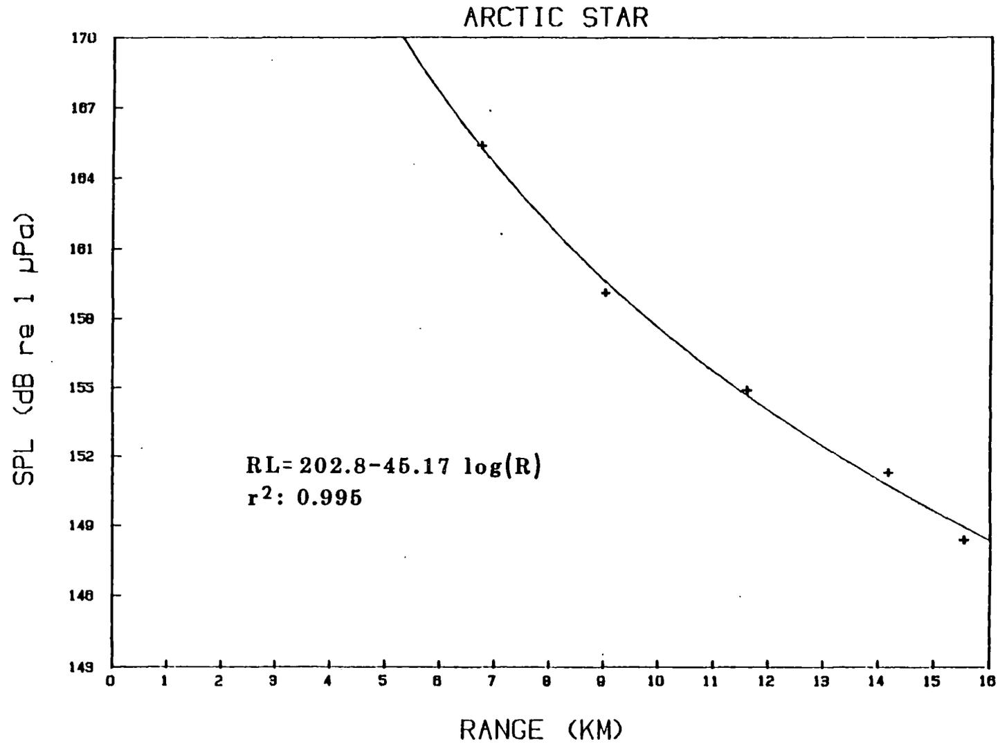
FIGURE 15. Arctic Star seismic level vs. range (logarithmic curve fit: RL = receive level, R = range in kilometers,  $r^2$  = coefficient of determination).
