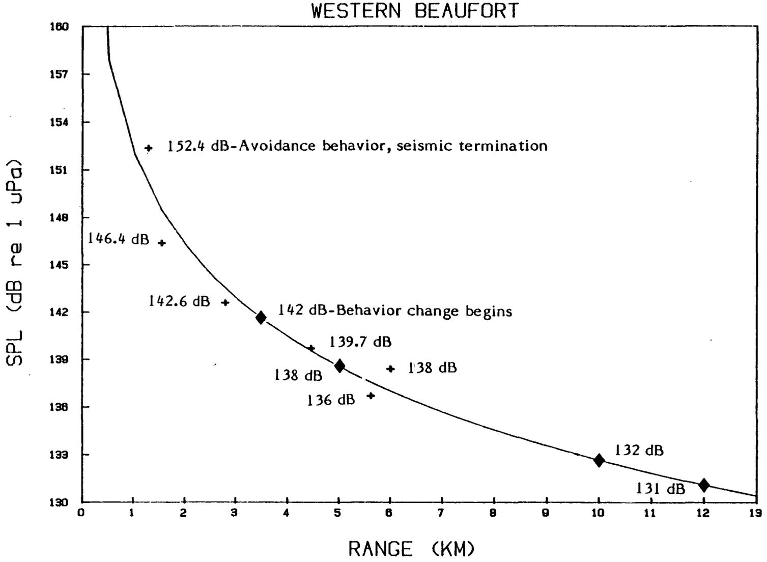
Figure 9. Received seismic sound levels versus range for the Western Beaufort. Line is a least squares regression line fit to the measured sound levels. ◆ = Estimated sound level; + = Measured sound level.
