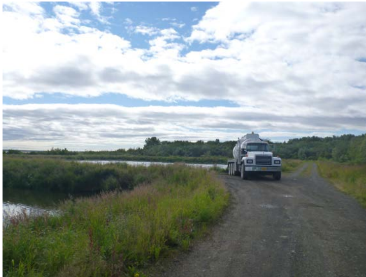
Figure 4. A septic system pump truck deposits anaerobic waste into the City of Dillingham’s aerobic sewage lagoon. The wastewater outflow from this lagoon repeatedly fails to meet water quality standards.
