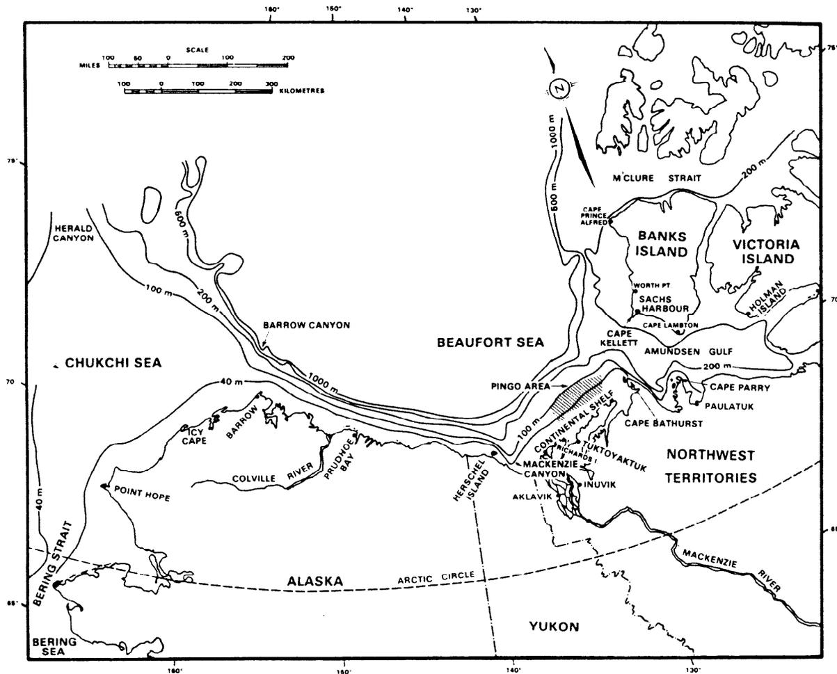
**FIGURE 1.4-2** Coastal bathymetry of the Beaufort Sea and Amundsen Gulf. In winter and spring most favourable ice conditions for Arctic tankers in the southeastern Beaufort Sea would be in a routing close to the 30 m isobath within the seasonal ice zone beyond the landfast ice edge. A ten mile wide shipping corridor is currently being surveyed through the pingo area and within the seasonal ice zone.
