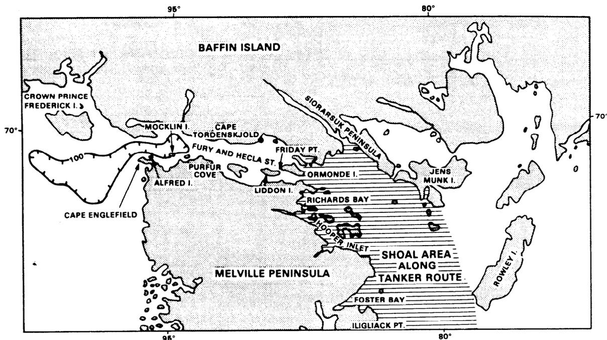
**FIGURE 1.4-7** Fury and Hecla Strait. Soundings have only been made through the centre of the strait and across a narrow section north of Purfur Cove. The strait is narrowest (1.95 km) between Ormonde Island and Melville Peninsula. During winter, the strait is mostly covered with first year landfast ice, however in summer, heavy ice can remain packed against the southern shore where water depths are greatest (Dickins, 1979).
