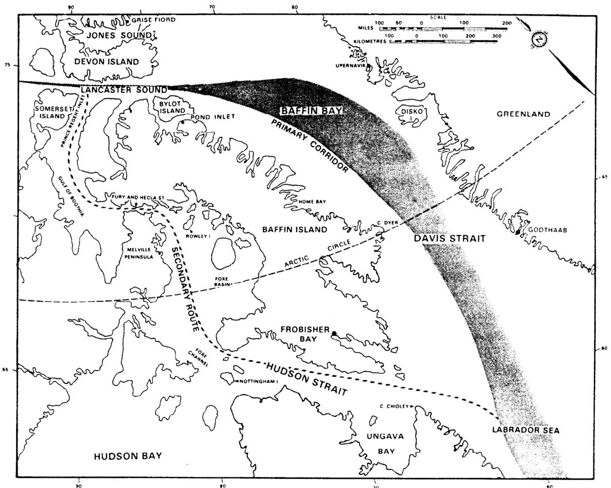
**FIGURE 1.1-5** The primary tanker corridor in Baffin Bay and Davis Strait. A secondary route (for smaller vessels) is through Prince Regent Inlet, Fury and Hecla Strait and Hudson Strait. This secondary route requires a more comprehensive set of soundings to determine whether or not it is a useful alternative.
