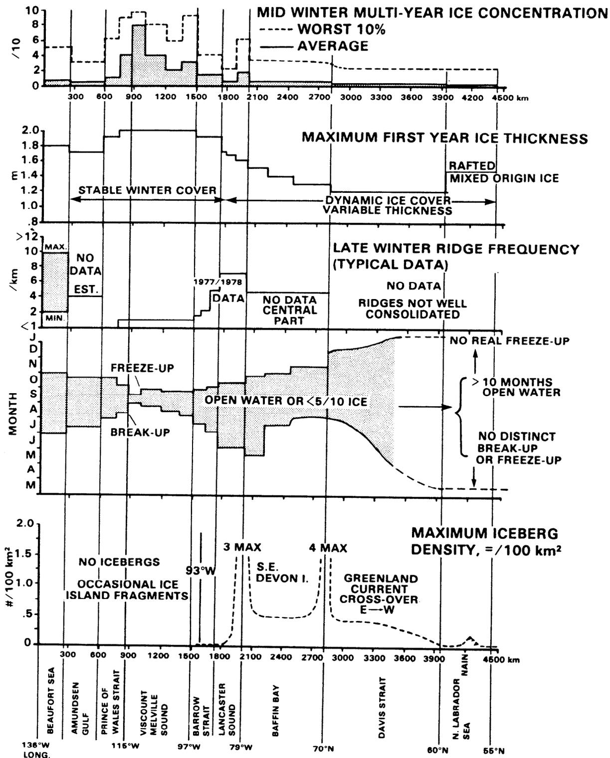
FIGURE 1.1-1 Ice conditions from the Beaufort Sea through to the North Labrador Sea (Source: Dickins 1978). The worst ice conditions are experienced in Viscount Melville Sound and the northern exit of Prince of Wales Strait.
