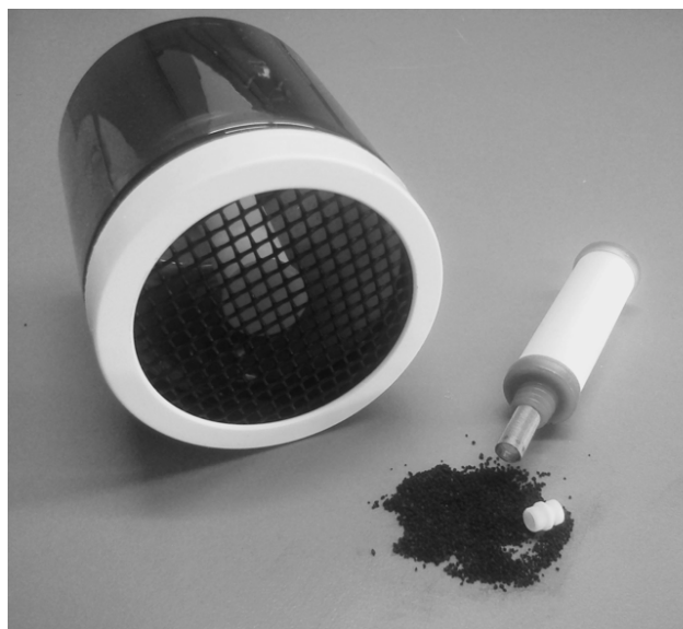
Figure 1. Mercury PAS Prototype - activated-carbon sorbent filled mesh cylinder inside a white Radiello® diffusive body.
