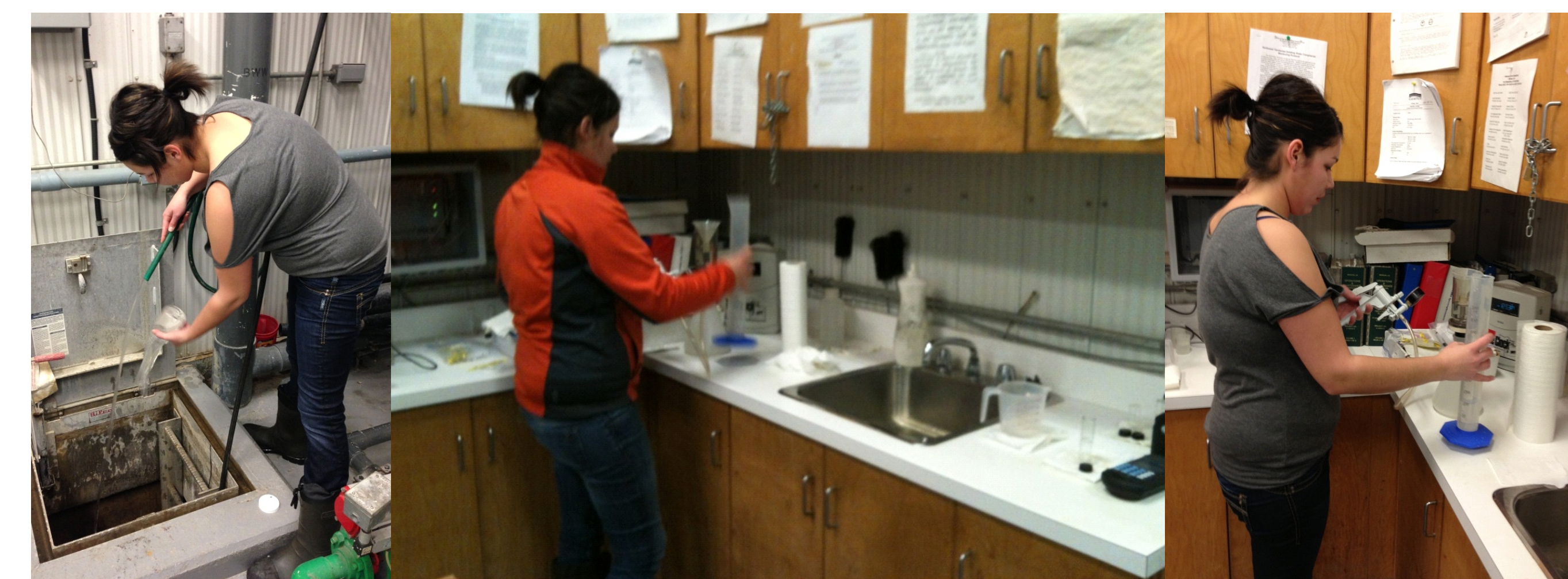
Figure 6. Elizabeth collecting, measuring, and filtering water for chlorophyll analyses in the water treatment plant laboratory.
