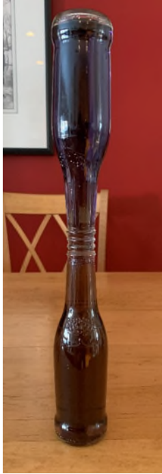
Figure 1: The cold water jar was placed on top of the warm water jar, causing a convection current where the lighter hot water rose as the heavier cold water sunk. This caused the two to mix, as visualized with the colours.
