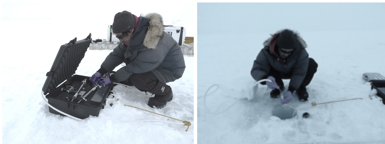
Figure 1. Sampling photos from May 2014: Right: Setting up the high volume pumping system and XAD column. Left subsampling for water chemistry from the pump outflow.
