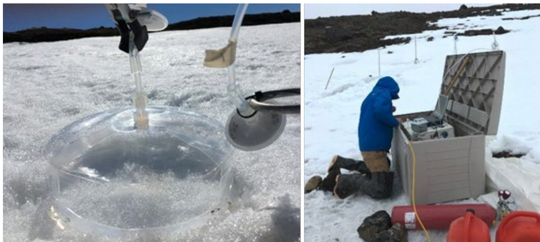
Figure 1. Photos from the spring 2017 field season including the Teflon DFC place over the late-lying spring snowpack (left) and project team member Chris Eckley checking the data stream of the Tekran 2537 (right).
